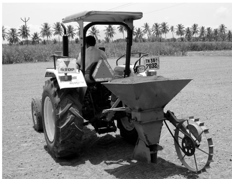
**Fig. 2** Operational view of subsoil coir pith applicator
