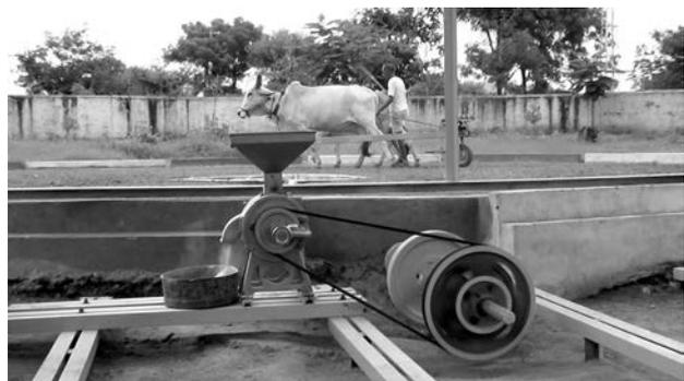
developed by Central Institute of Agricultural Engineering, Bhopal (India) was used to vary the load on the system. A loading car was attached with the help of chain and sprocket (Fig. 5) and load was varied by regulating the hydraulic valve of the loading car. A load cell was attached between horizontal pull beam and animal hitching system to measure the actual load on the power transmission system (Fig. 4).
