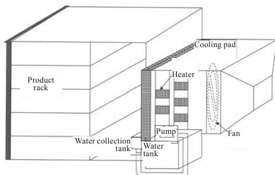
**Fig. 2** Betel leaf conditioning chamber (inside and outside view)
