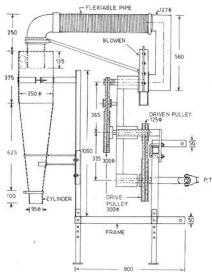
**Fig. 2** Front elevation of experimental picking aid (all dimensions are in mm)
