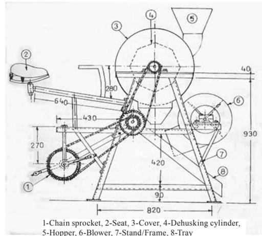
**Fig 7** TNAU Maize Dehusker-sheller
