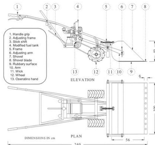
fied reaper are indicated in **Table 1**. Moreover, a diagram of the experimented shovel and a geometrical drawing of the modified reaper are illustrated in **Figs. 1** and **2**, respectively. The suggested modification in this study was fulfilled in one of the workshops at the Industrial City, Kafr Elsheikh Governorate.
