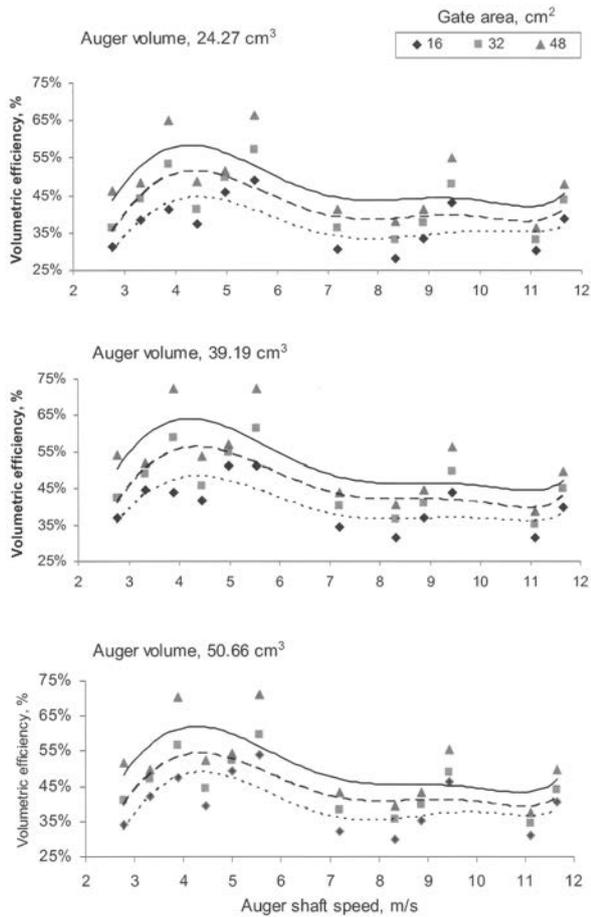
**Fig. 8** Effect of auger shaft speed on volumetric efficiency for Urea
