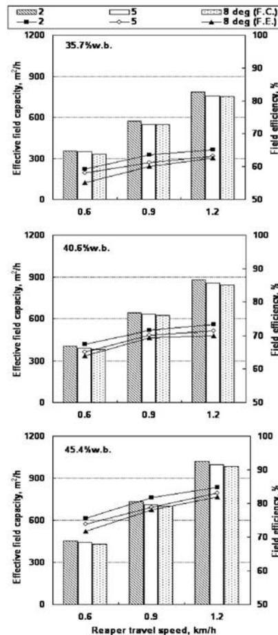
**Fig. 6** The variation of litter removal efficiency as affected by reaper travel speed at different levels of litter moisture content and shovel blade tilt angle
