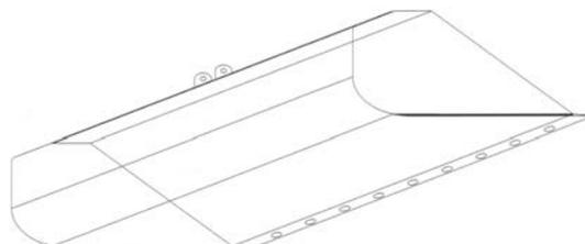
**Fig. 2** A perspective of the alternative broiler litter removal system (the modified reaper)
