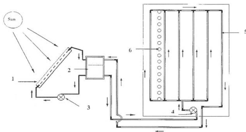
1. Solar collector, 2. Insulated storage tank, 3. and 4. Water pumps, 5. Heat exchanger, and 6. Cucumber pots
