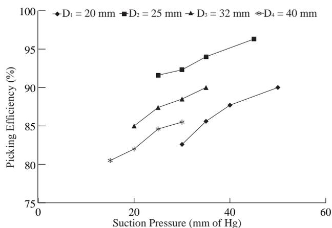
Fig. 4 Extrapolation of trends of picking efficiency
