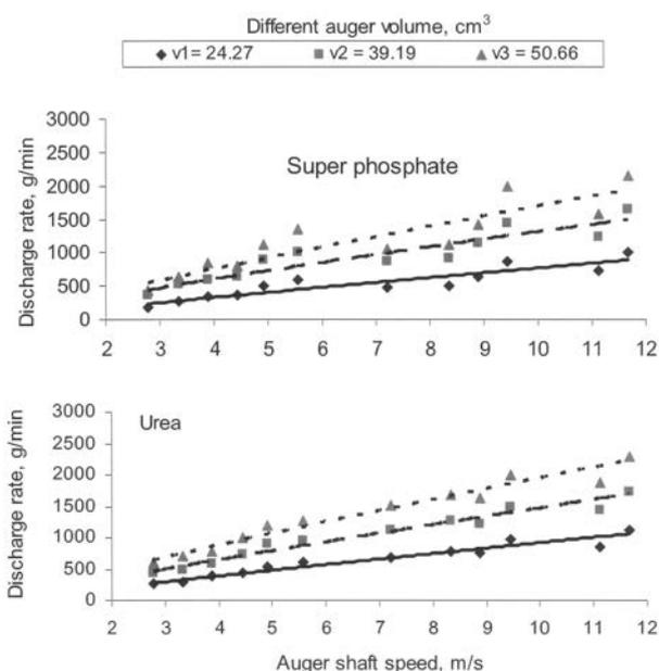
Fig. 5 The discharge rates of fertilizing metric device at the gate area of  $32 \text{ cm}^2$
