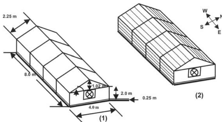
1. Covered with corrugated fiberglass reinforced plastic,
