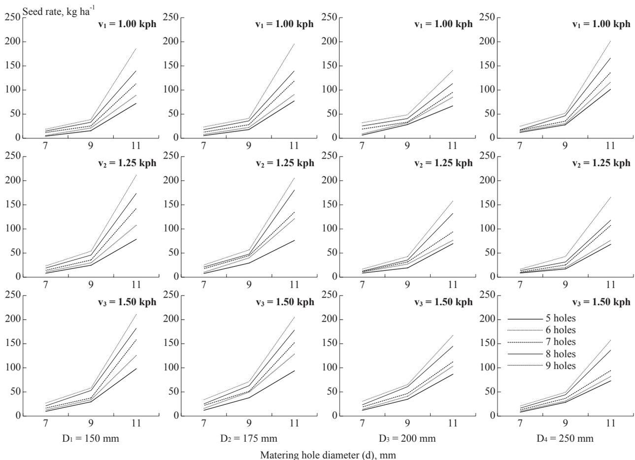
Fig. 6 Effect of hole diameter on seed rate at selected forward speed of operation for cylindrical ellipsoid drum (S<sub>3</sub>)
