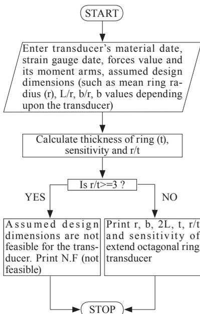
Fig. 3 Flow chart for simulation of extended octagonal ring transducer design program
