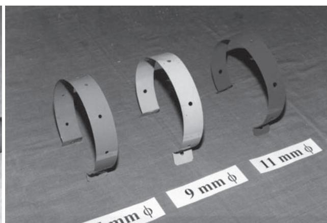
Fig. 2 Strips with varying diameter of seed metering holes
