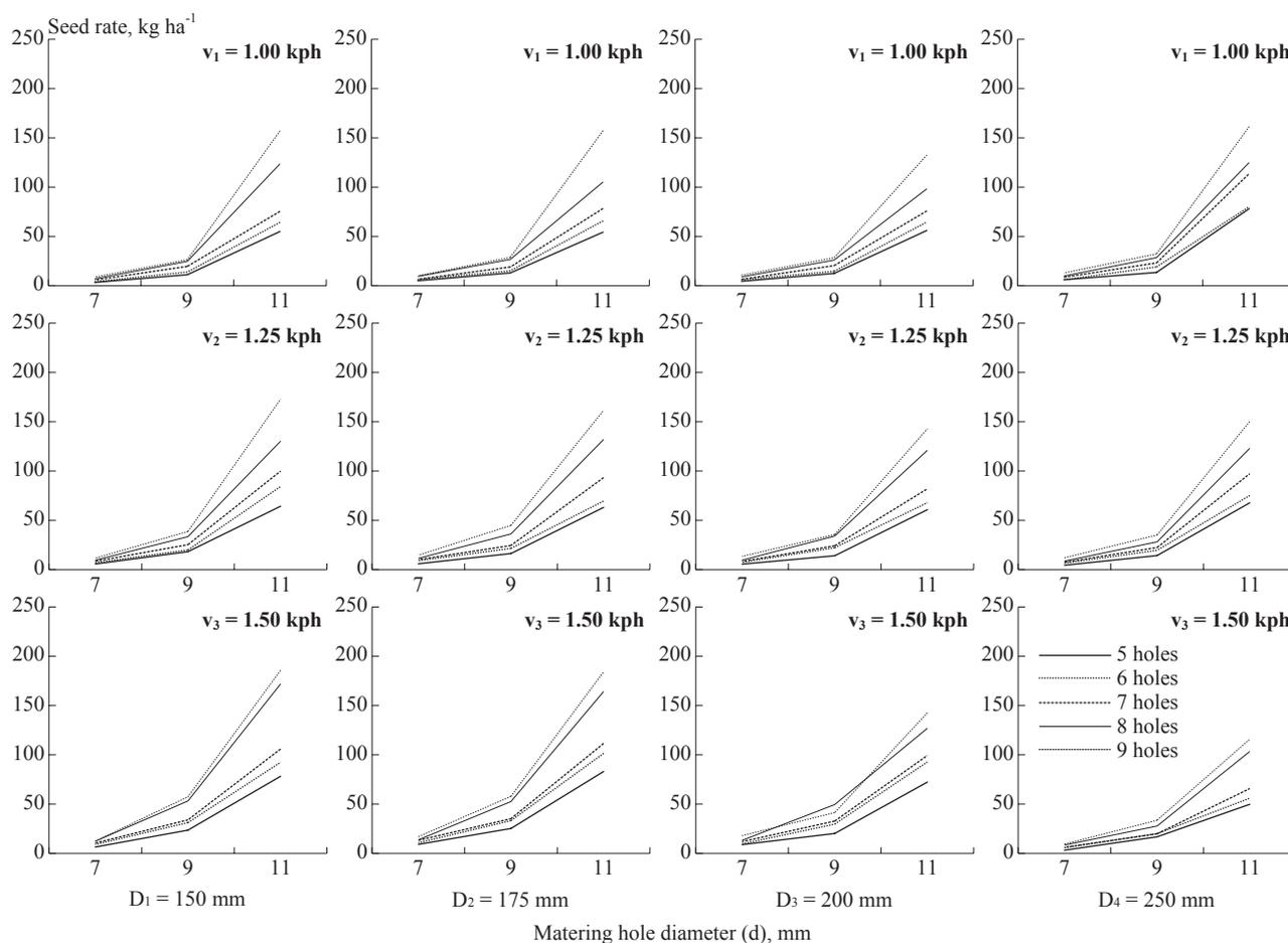
Fig. 4 Effect of hole diameter on seed rate at selected forward speed of operation for cylindrical drum (S<sub>1</sub>)
