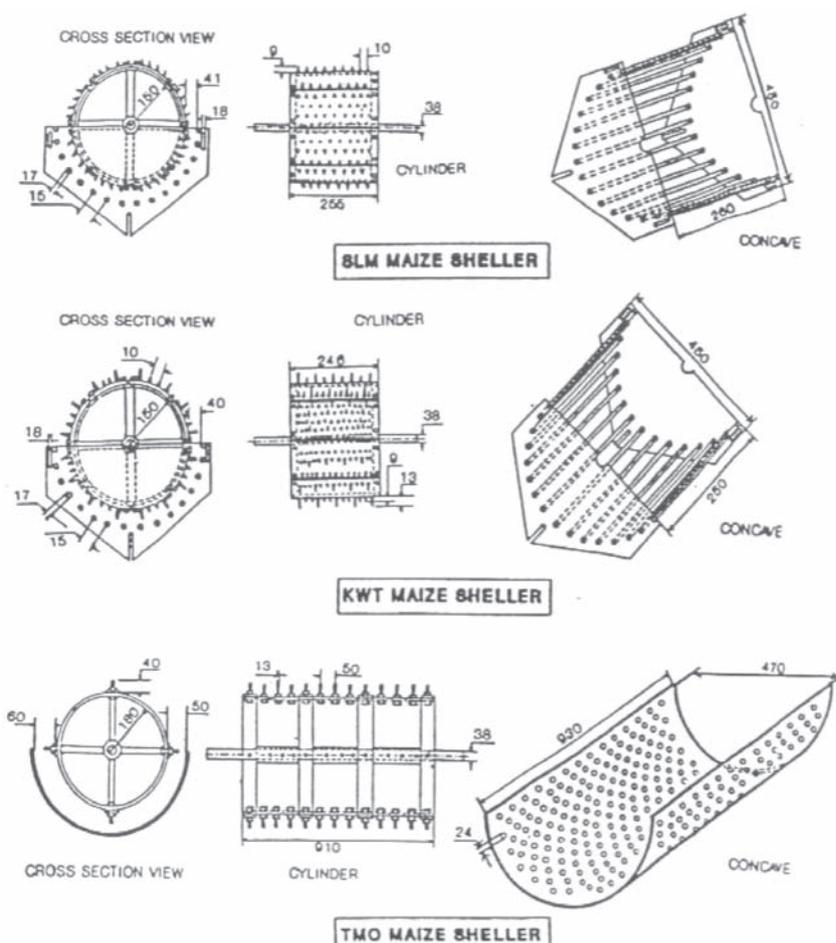
**Fig. 2** Schematic diagram of the cylinder and shelling concave of the three local maize shellers
