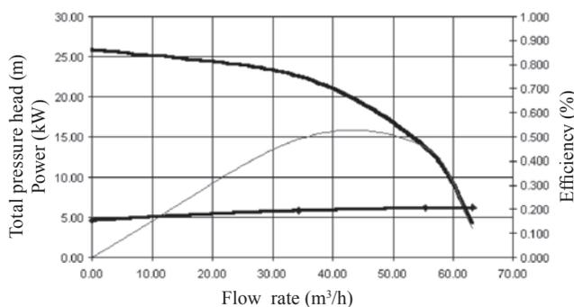
Fig. 9 Pump characteristics for open type pump with cast iron impeller
