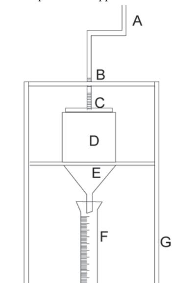
A: Handle, B: Ram, C: Plunger, D: Compression chamber, E: Funnel, F: Measuring cylinder, G: Frame
