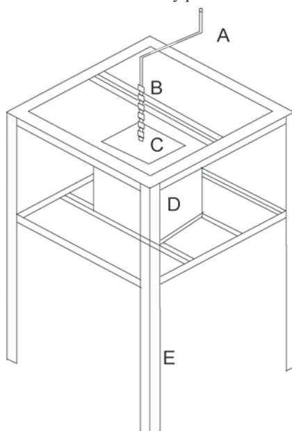
A: Handle, B: Ram, C: Plunger, D: Compression chamber, E: Frame
