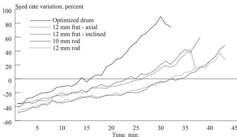
Fig. 9 Percent variation in seed discharge of the prototype drum seeder with different types of baffles
