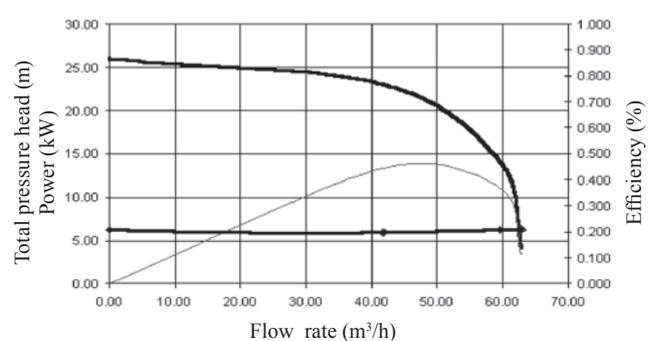
Fig. 10 Pump characteristics for open type, cast brass impeller pump
