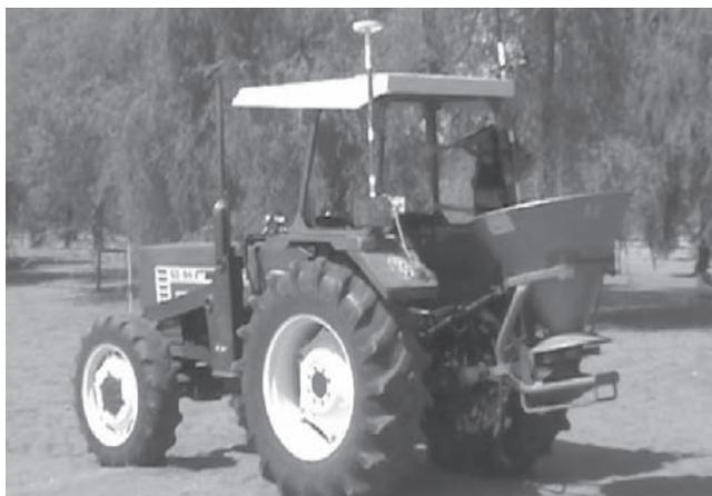
Fig. 4 The semi-automatic VRT spreader
