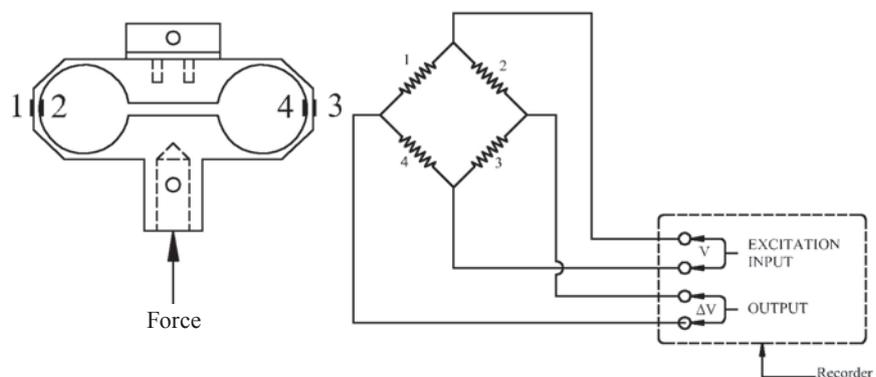
**Fig. 5** Transducer and circuit diagram for measurement of forces
