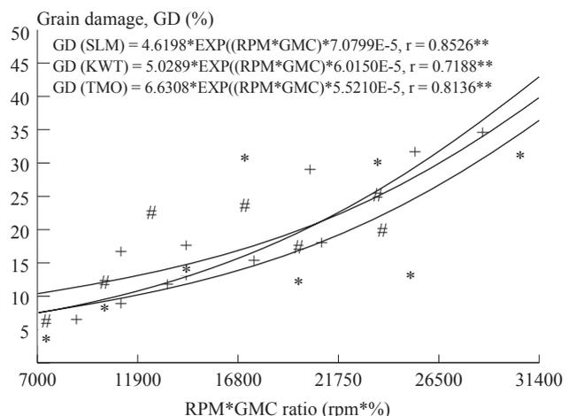
Fig. 4 Effect of cylinder speed and grain moisture content on grain damage for three types of maize sheller (+ SLM, \* KWT and # TMO)
