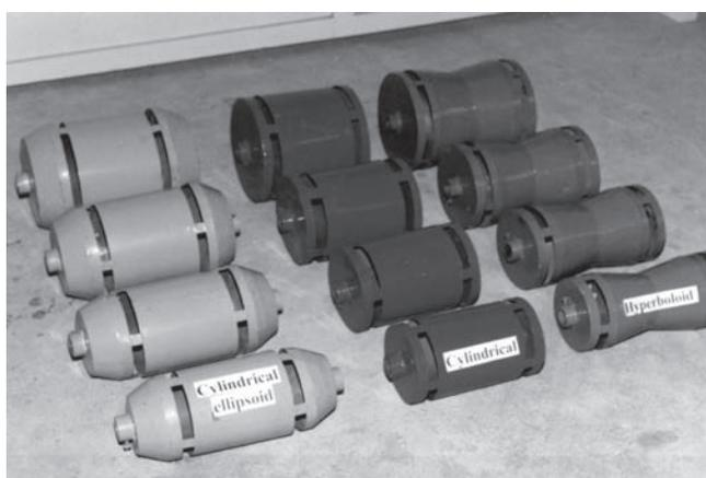
Fig. 1 View of selected seed drum shapes (150, 175, 200 and 250 mm diameter)
