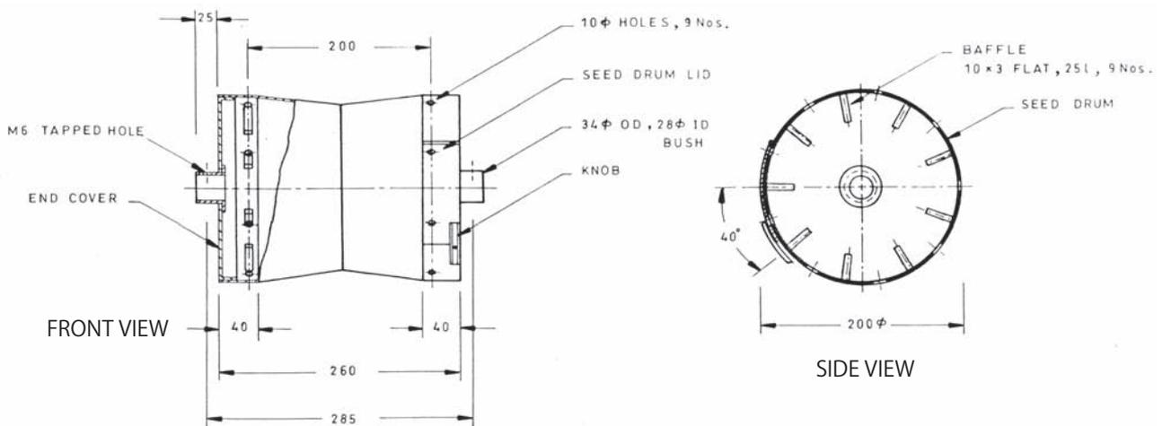
Fig. 3 Hyperboloid seed drum with baffle arrangement
