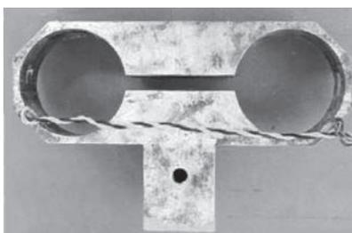
**Fig. 4** The extended octagonal ring transducer fabricated based on simulation
