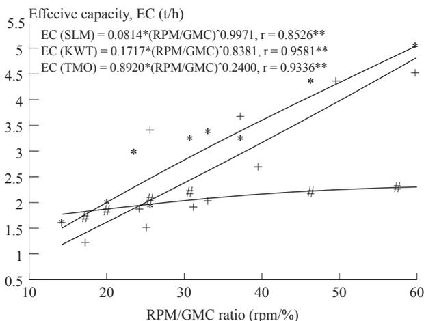
Fig. 3 Effect of cylinder speed and grain moisture content on effective capacity for three types of maize sheller (+ SLM, \* KWT and # TMO)
