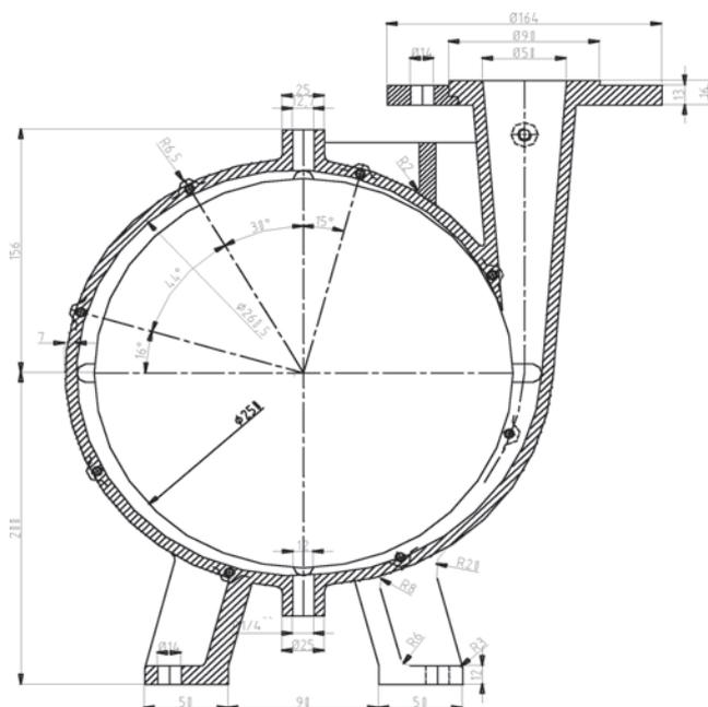
**Fig. 1** Body of centrifugal pump with the closed impeller
