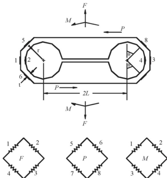
Fig. 1 Extended octagonal ring transducer with strain gauges for measurement of forces and moments
