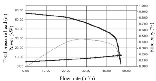
Fig. 8 Pump characteristics of close type, cast iron impeller coated with polymer composite materials
