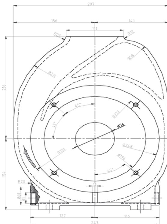
**Fig. 2** Body of the centrifugal pump with open impeller
