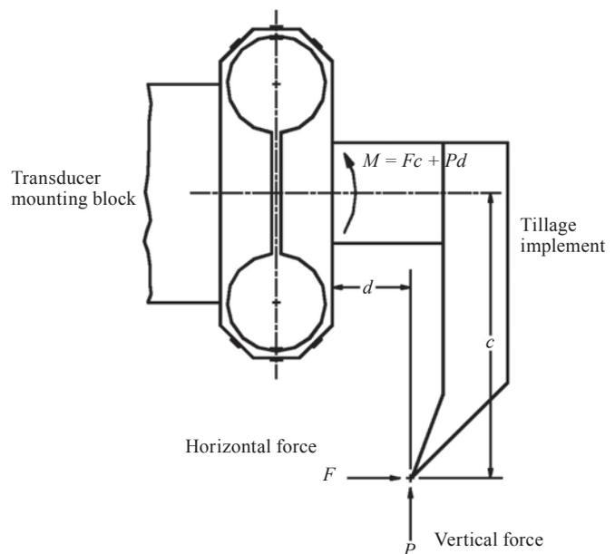
Fig. 2 Forces acting on a soil tillage implement attached to the extended octagonal ring transducer and their resulting moments
