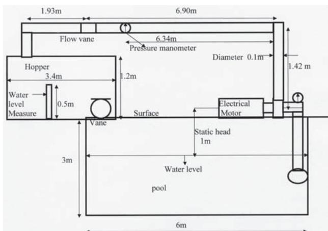
**Fig. 5** Pump testing apparatus
