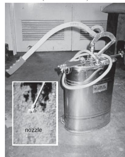
**Fig. 2** The designed LOK sprayer
