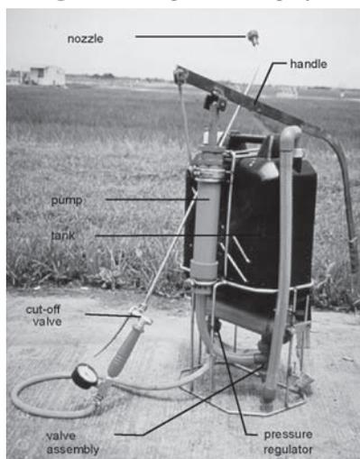
**Fig. 3** The prototype's pressure regulator
