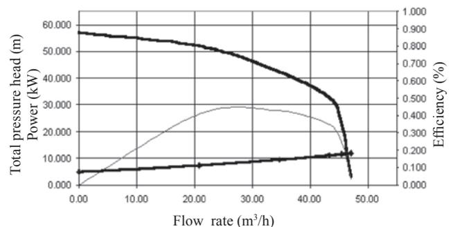
**Fig. 6** Pump characteristics of the cast iron impeller
