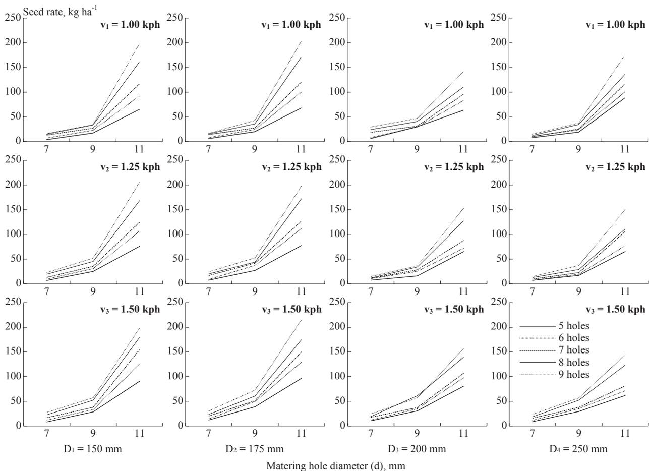
Fig. 5 Effect of hole diameter on seed rate at selected forward speed of operation for hyperboloid seed drum ( $S_2$ )
