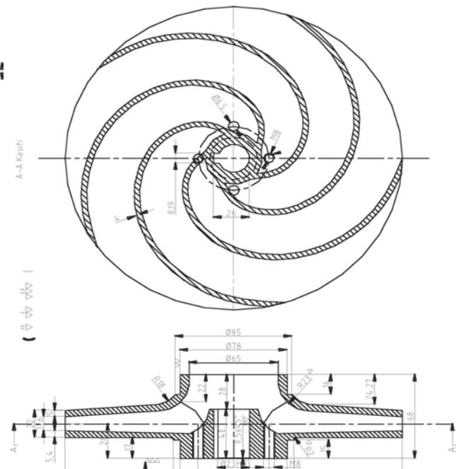
**Fig. 2** Closed impeller
