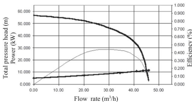
Fig. 7 Pump characteristics of the cast brass impeller
