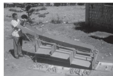
**Fig. 2** Raw mango grader
