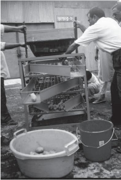
**Fig. 2** Potato grader in operation
