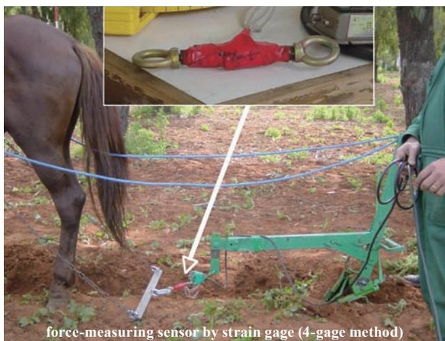
force-measuring sensor by strain gage (4-gage method)
