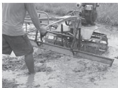
Fig. 8 The spring-activated PhilRice leveler
