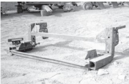
**Plate 2** A combined differential chassis
