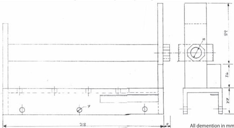
Fig. 3b Power regulating unit part 2
