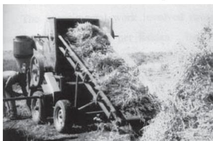
Fig. 1b The cyclone vines collector
