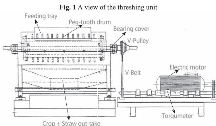
1980). Increasing the V and the C raised the power consumption because of the positive coefficient value. The power requirement of the drum increased with drum speed because of the increased feed rate, which accounted for the extra energy required for threshing material. The increasing feed rate required greater compression of the material as it passed between the threshing drum and concave and caused an increase in power requirement (Sudajan et al., 2002).
