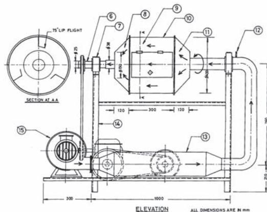
1. Reduction gear box, 2. Motor, 3. Hollow shaft, 4. Heating coil, 5. Insulator, 6. Exhaust pipe, 7. Bearing, 8. Exhaust chamber, 9. Drying chamber, 10. Rotary drum, 11. Plenum chamber, 12. Thermocouple, 13. Heating chamber, 14. Main frame, 15. Blower
