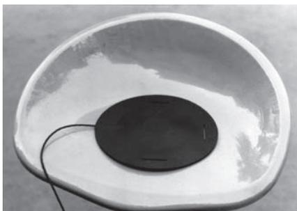
**Fig. 3** Triaxial seat accelerometer placed on the trailer seat
