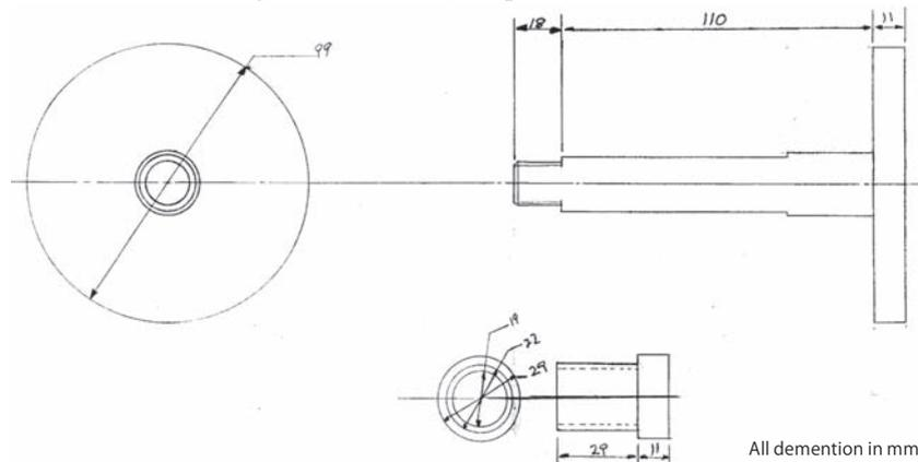
**Plate 4** The modified universal joint
