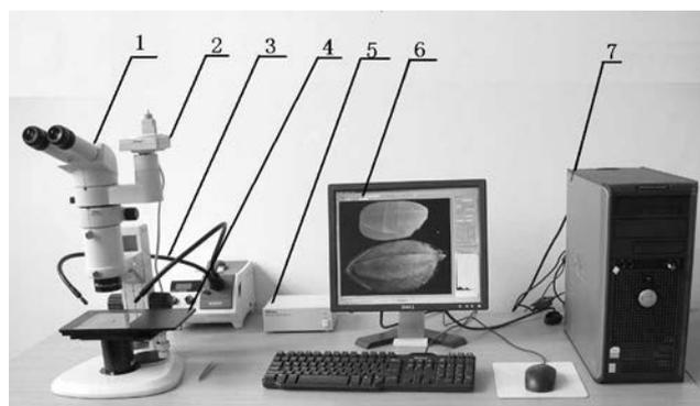
1. Stereo microscope 2. CCD camera 3. Light source 4. Removable platform 5. Controller 6. LCD screen 7. Computer host
