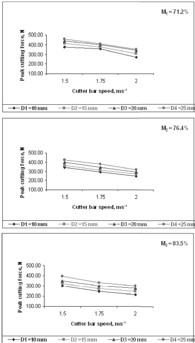
**Fig. 6** Effect of cutter bar speed on peak cutting force at selected levels of diameter and moisture content of maize stalk for 90.0 mm stroke length of cutter bar ( $L_2$ )
