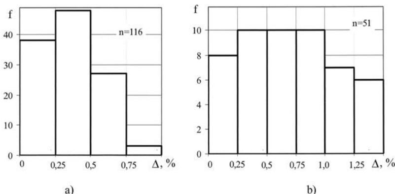
**Table 1** Statistical estimation of absolute error of moisture measurements with the “Aquasearch PM-600”
