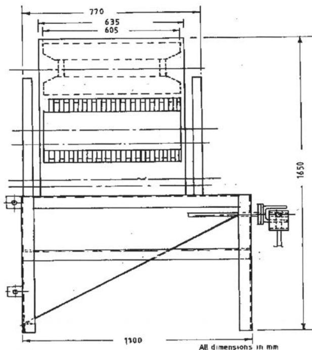
Fig. 2 Schematic view of sugarcane cleaner (front view)
