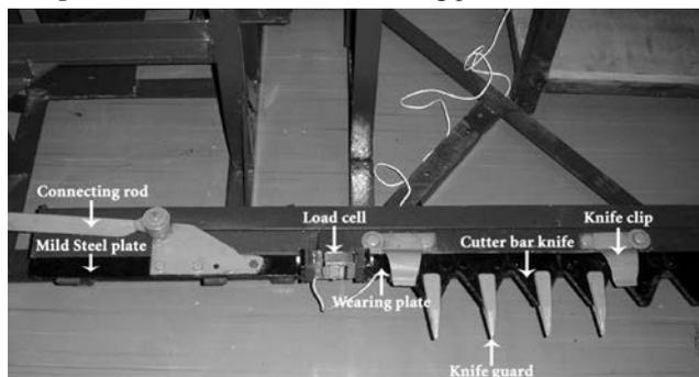
obtained by subtracting the inertial forces and frictional force of idle reciprocation from the gross dynamic cutting force. The force calculated for each position of the cutter bar was plotted as a force - distance curve as shown in Fig. 3. The peak cutting force (PFC) required for harvesting the selected maize fodder crops was recorded for all treatments.
