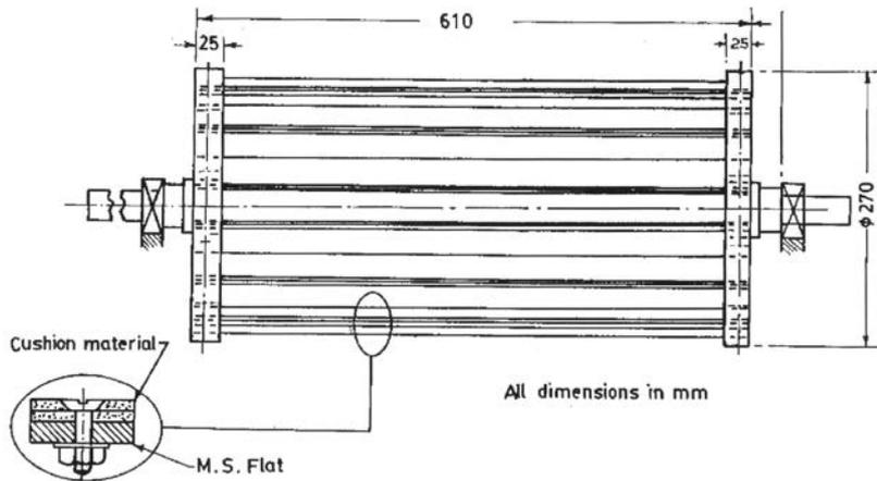
**Fig. 4** Blower of tractor-operated sugarcane cleaner
