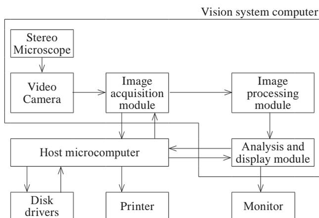
Fig. 3 Computer vision instrument for detecting stress cracks in rice kernels
