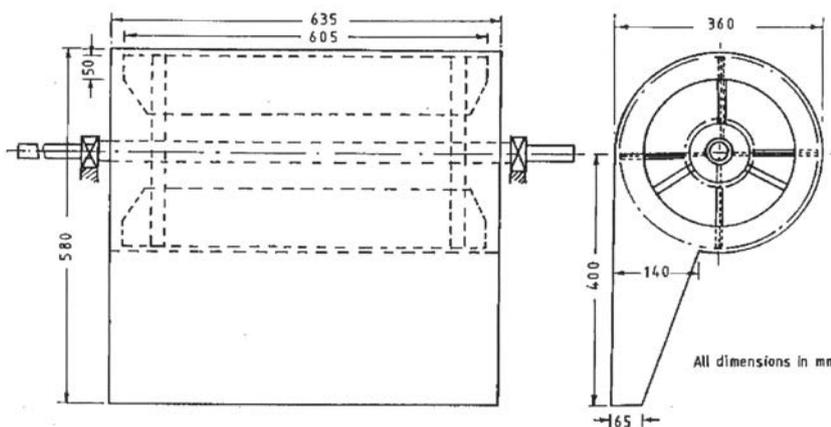
**Fig. 5** Flap roller of tractor-operated sugarcane cleaner
