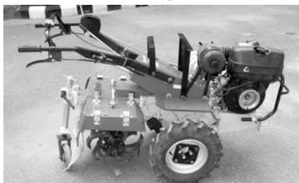
Fig. 2 Oleo power weeder
