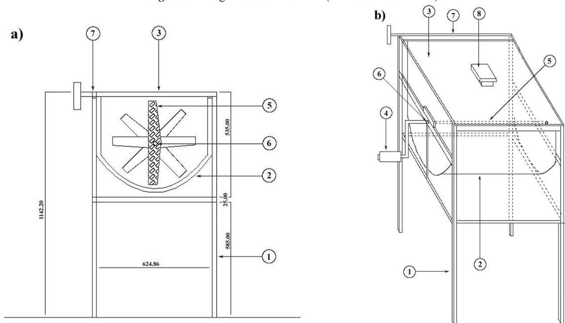
1. support structure, 2. churner chamber, 3. churner chamber cover, 4. handle for hand operation, 5. baffled shaft, 6. bearings, 7. hinge, 8. handle for emptying the chamber cover
