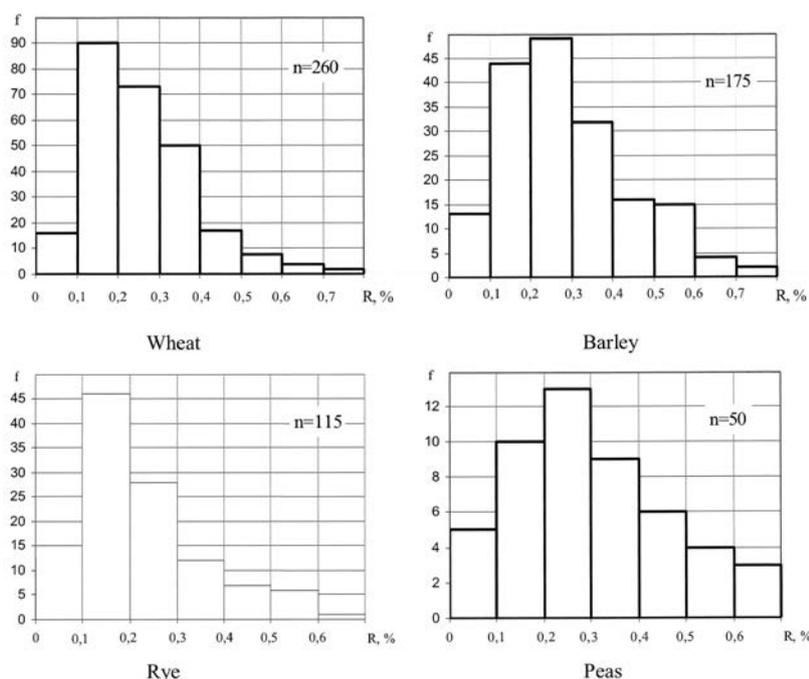
**Table 2** Estimation of convergence of moisture meter measurements for grain of eared and leguminous crops
