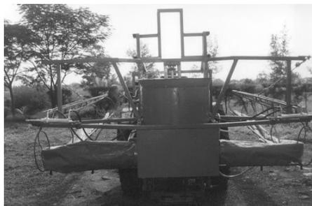
Fig. 8 View of folder air sleeve boom to facilitate transportation
