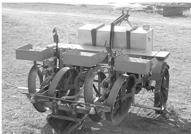
**Fig. 2** An isometric view of tractor operated two-row vegetable transplanter
