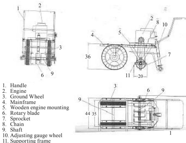
**Fig.2** Schematic diagram of short handle hoe
