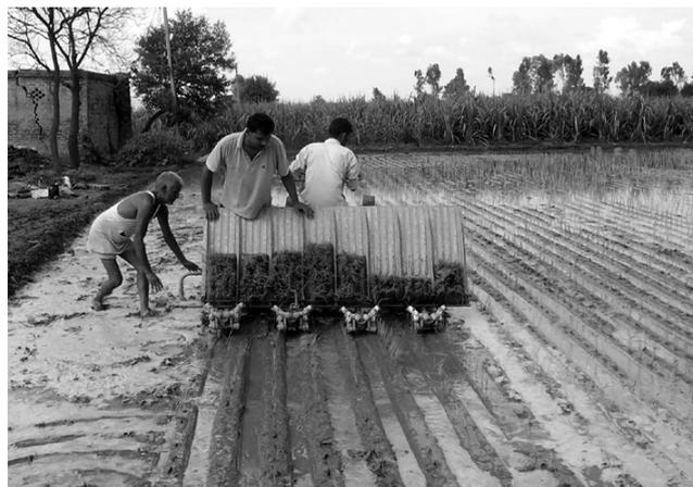
Fig. 4 Mate type seedling growing for self-propelled rice transplanter
