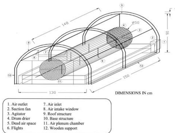
**Fig. 3** Working principle of the greenhouse solar drier during loading and unloading sugar beet tops
