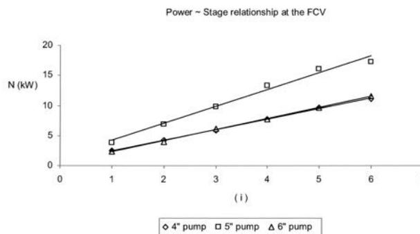
depending on the stage number ( $R^2 = 0.6743 \dots 0.9711$ ). Increased rates of the efficiencies were 10, 32 % -19 and 50 %.
