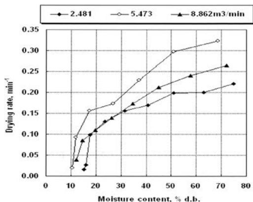
Fig. 12 The variation of drying rate as a function of moisture ratio at several airflow rates
