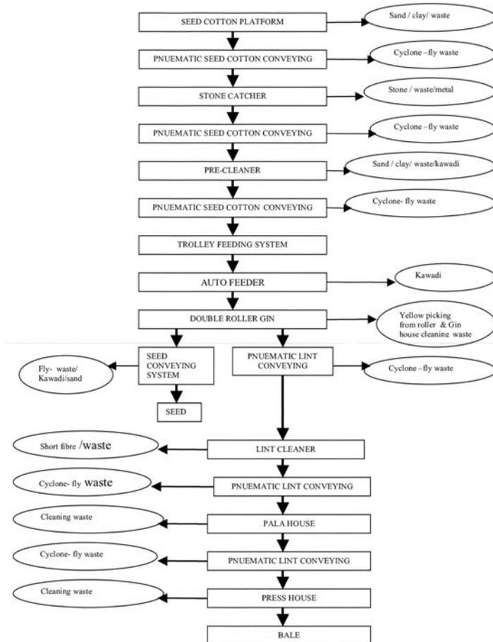
**Fig. 1** Schematic diagram depicting the sequence of machinery used in cotton processing in a modernized gin
