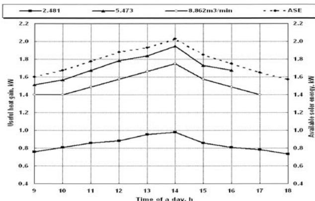
Fig. 8 Solar drier thermal efficiency versus time of day at various airflow rates
