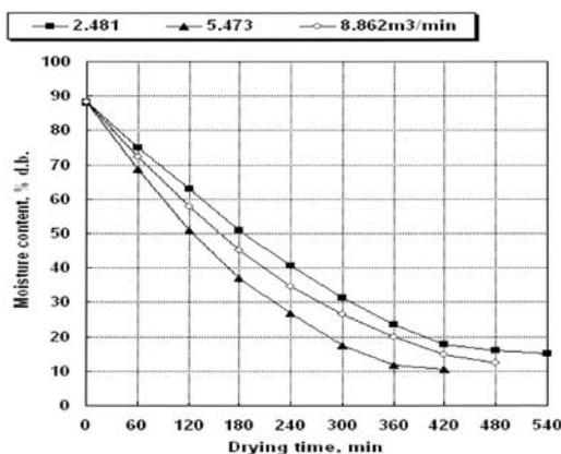
**Fig. 10** Variation of moisture ratio with drying time of sugar beet tops at several airflow rates
