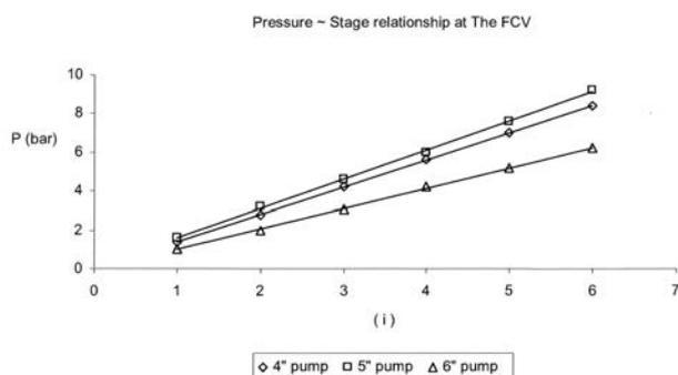
**Fig. 2** The effect of stage number on power for the multistage deep well pumps
