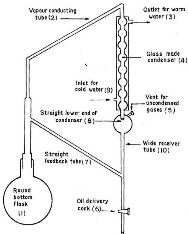
Fig.3 Schematic diagram of Betel leaf oil extractor
