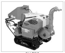
KARUI Chipper "DraCom KDC-131B" Grind the branches in parks, bamboo woods, and fruit farms into useful woodchips and decrease the volume at the same time. ■L1800×W770×H1250 mm ●415kg ▲9.6kW □Max. branch: ø120mm □Processing Capacity: 800-1300kg/h
