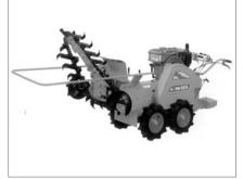
KAWABE Trencher for Multi-Crops "NF-843" By forward movement you can plow to replace surface soil with subsoil. ■L2150×W800×H1090mm ●297kg ▲Water-cooled Diesel 8ps □Tire: 4.00×8AG □4 wheel driving vehicle with same Dia. tires. □Self propelled
