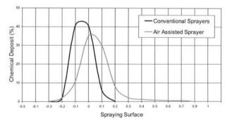
Fig. 5 Spray distribution curves for conventional and air assisted sprayers
