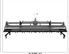
NIPLO Rotary Harrow "HL4020B" High durability guaranteed by the double frame structure. Large spring-brake ploughs in the straws and residual stems beautifully. L850×W4150×H1395mm •575kg Å70-100ps □Working Width: 391cm □Side drive
