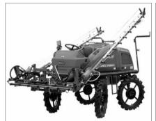
MARUYAMA Boom Sprayer "BSA650LDE" For crop management in rice paddy and field cultivation. ■L3940×W2150×H2400 /800mm (effective ground height) ●1145kg ▲15.4kW, 1123cc □Discharge Rate: 100L/min DWorking Width: 9.9-15.9m
