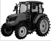
**ISEKI** *Tractor "TJV95"* High output and torque engine of 95ps equipped. Common rail type electronic fuel injection system applied. This tractor computerizes the fuel injection, and the user is able to choose from two types of engine output patterns "Output Priority Mode" and "Fuel Consumption Priority Mode".
