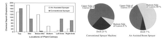
air effect to separate the leaves of plants so that the atomized chemicals could be deposited on both upper and under sides of the leaves.
