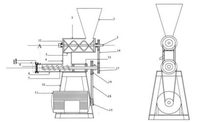
1: Hopper, 2: Conditioner Shaft, 3: Conditioning Chamber, 4: Feeding Channel, 5: Shutter, 6: Screw Press barrel, 7: Screw Press, 8: Die, 9: Die Holder, 10: Frame, 11: Electric motor 12: Conditioner Shaft Bearing, 13: Screw Press shaft Bearing, 14: Screw Press pulley, 15: Electric Motor Pulley, 16: Driven Pulley of Conditioner, 17: Driver Pulley of Conditioner, 18: Screw Press Belt Drive, 19: Conditioner Belt Driver
