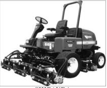
SHIBAURA Reel Mower "SR525A-S" Lightweight Quintupulex. One of the best-in-class lightweight and full fledged, compact and underslung machine. ■L2700×W2900×H2040mm ●1320kg ▲27.9kW/2850rpm, 1662cc □HST □Working Width: 2500mm
