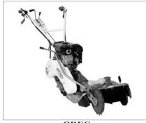
OREC Dehedral Levee Bush Cutter "Wing Mower WM624A" ■L1785×W830×H940mm •61kg ▲4.3 hp □Handle load: 9kg □Speed change: F2, R1 □Driving wheels: F □Working Width: 600×H10-70mm (left roter adjustable in 4 levels) □4 bar knives
