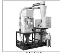
SATAKE Mill "SRG30A" Rice Powder Food Responded Flouring Machine. Able to flour from small amount. ■W1950×D1000×H2896mm □Processing Ability: 30kg/h □Required power: 3-phase 200V 8.55kW
