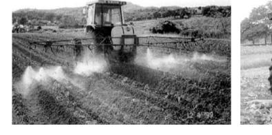
tato pest and disease management (**Fig. 5**). Both single and double-row planting is the best for the sprayer in terms of speed of operation and savings in chemicals. With a machine, spraying height and angle can be controlled according to the height of the crop from the ground and the canopy structure. With the help of a tractor pto shaft, chemical droplets can penetrate deep into the canopy preventing insects from breeding inside the dense canopy.
