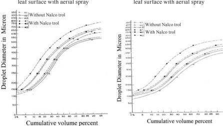
Fig. 3 Droplet size distribution of upper leaf surface with aerial spray
