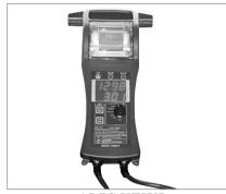
ALPS KEIKI Battery Tester "SP1250BT" Applying "Kinetic Inward Resistance System" (patent), which estimates the ohmic value by looking at the displacement of current and tension in the battery while charging and discharging. ■L145×W280×H70mm • 800g
