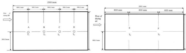
Fig. 3 Arrangement of thermocouples for sensing moist air temperature just above the agricultural materials
