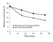
Table 3 Moisture content readings obtained during drying of paddy rice
