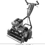
SHIBAURA Green Mower "G-EXE" The perfect finish for a variety of greens. ■L1100×W970/1055×H1050mm •78/83kg ▲3.2kW/4,000rpm, 2700cc □Working Width: 557/643.5mm □Mowing speed: 4.3/5.5 □Cut frequency stages: 3.5/4.5/5.1/6.5mm □Off-set moving system (5 settings from 4-12mm)
