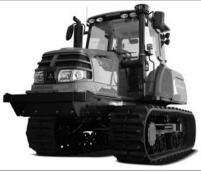
**MITSUBISHI** Tractor "GCR1350" ■L4260×W2100×H2640mm ●5300kg ▲4-cycle, Water-cooled diesel 92.8kW/2200rpm, 4398cc □Crawler: W550×L2390mm □HST □PTO: 559, 793, 1040rpm
