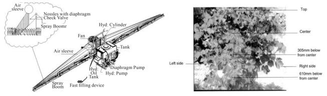
an inlet and outlet valves. Liquid was drawn through the inlet valve by movement of the diaphragm and, on the return of the diaphragm, was forced out through the outlet valve. The pump was located at the rear of the spraver frame for easy service and maintenance and delivered 80 L/min of chemical at a pressure of 40 bars.
