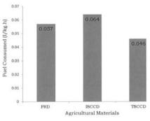
time of agricultural material dried. Drying of the threadlike shaped cassava chips gave the least fuel consumption rate of 0.046 l/kg.h. This was followed by paddy rice drying which gave a fuel consumption rate of 0.057 l/kg.h, and drying of irregular shaped cassava chips with the highest fuel consumption rate of 0.064 l/kg.h. This implied that the NCAM modified batch dryer was economical in drying the threadlike cassava chips as compared to the other two agricultural materials.
