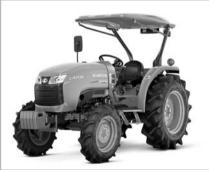
**KUBOTA** *Tractor "L4708"* L4708, is a high perforamnced L-series tractor which can be operated in both paddy and dry field with high horse power and column shuttle specification. **4**47ps
