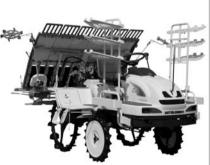
**MITSUBISHI** Rice Trans-Planter "LV63" ■L3255×W2000×H1930mm □Ground height: 435mm ●696kg ▲Water cooled 4-cycle, OHC gasoline. 16.0ps/2800 rpm □HST □Rotary type □Rows: 6  $\square$ Width of stub: 11/12/14/16/18/21cm
