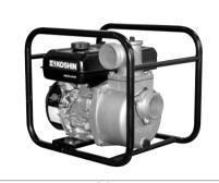
KOSHIN "Hidels Pumps SEV-80X" PUMP □Connection: 80mm □Total Head: 25m □Delivery Volume: 1050L/ min □Max. Suction Head: 8m ENGINE ▲3.1kW/3600rpm, 179cc •7.7kg
