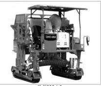
**OCHIAI** Riding Type Tea Picking Machine "OHC-6A" Full working width cutter bar. Stepless speed control. **A**Water-cooled Diesel engine 28.4ps.
