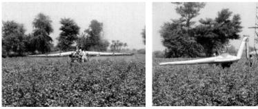
pipes  $20.3 \times 42$  mm with 13.5 mm inside diameter PVC pipe fitted inside the frame. The boom was made in five sections with a total width of 10.7 m and 20 nozzles with 510 mm spacing and two outer sections on both sides that were foldable. The boom height and its folding/unfolding were controlled through hydraulic cylinders operated through a hydraulic pump.
