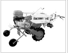
**MAMETORA** Vegetable Transplanter "**TP-4**" This machine is available both pot and soil block in seeding transplanting. ■L217×W122×H106-130cm •170kg ▲4.4ps/2000rpm, 126cc □Speed: 0.2-0.4m/s  $\Box$ Efficiency: 10a/1.5-2.0h  $\Box$ Rows:
