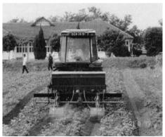
Fig. 3 Tractor-mounted single-row planter
