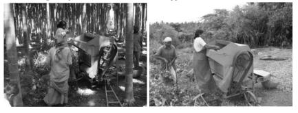
Fig. 5 Operational view of arecanut sripper with men workers
