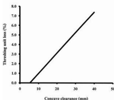
**Fig. 8** Effect of side concave clearance on threshing unit loss
