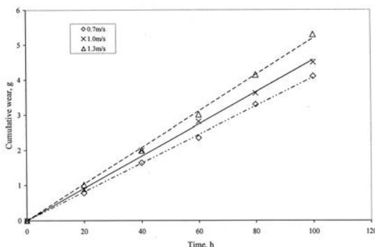
Fig. 4 Effect of speed on wear rate of shovels
