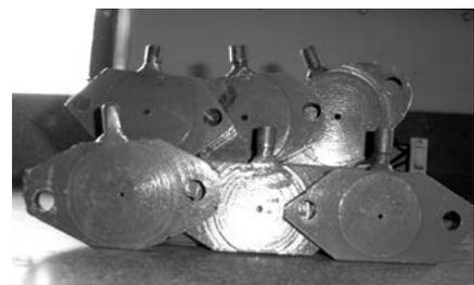
The equipment studies were conducted to determine the injection rate through the different sizes of the orifice meters. After preparing the fertilizer solution, the water flowing through orifice meter was applied to the area under fertigation. All developed equipment were tested under various inlet discharges and rates of fertilizer injection. All orifice meters were tested for areas 450 m<sup>2</sup>, 300 m<sup>2</sup> and 150 m<sup>2</sup>
