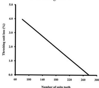
**Fig. 11** Effect of height of spike teeth on threshing unit loss
