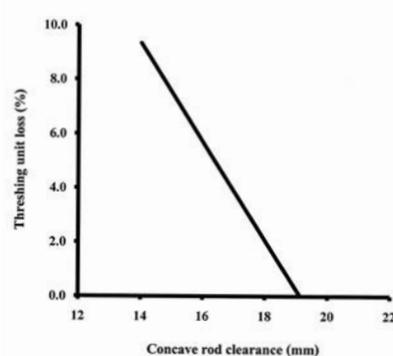
**Fig. 7** Effect of concave clearance on threshing unit loss
