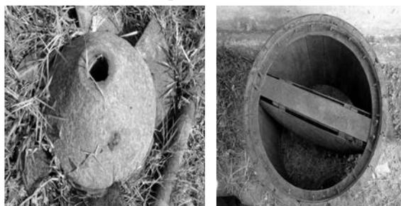
the Para is provided with a butterfly mild steel foot valve for restricting the backward flow as shown in **Fig. 3b**. The foot valve is seated perfectly over the M.S. ring without any leakage in order to avoid priming of the pump often. The views of a typical Petti and Para are shown in **Fig. 4**.
