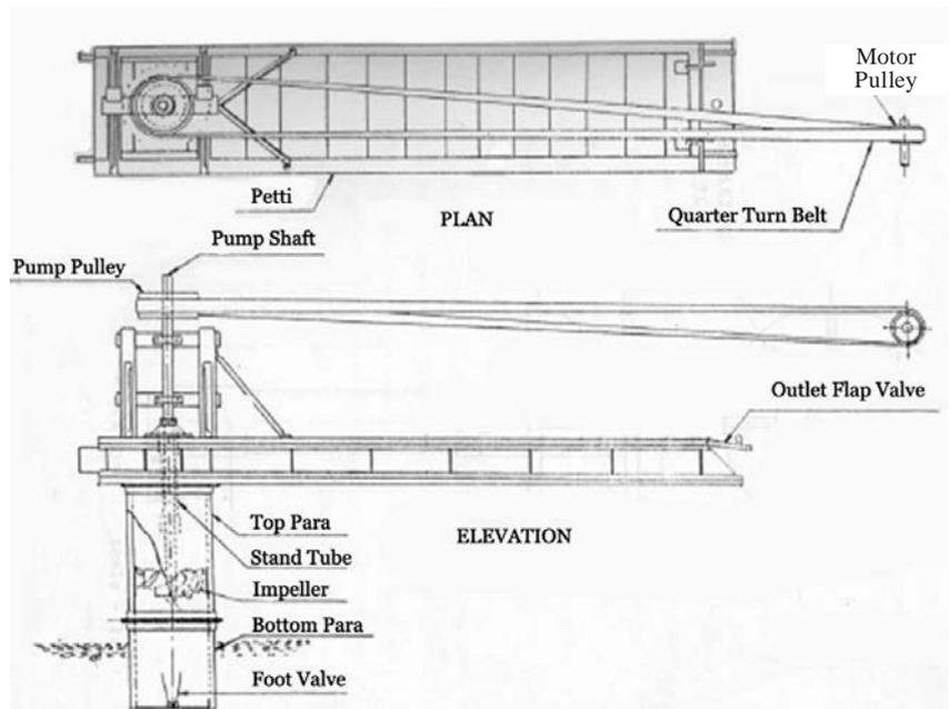
**Fig. 5** Portable axial flow pump (IRRI)
