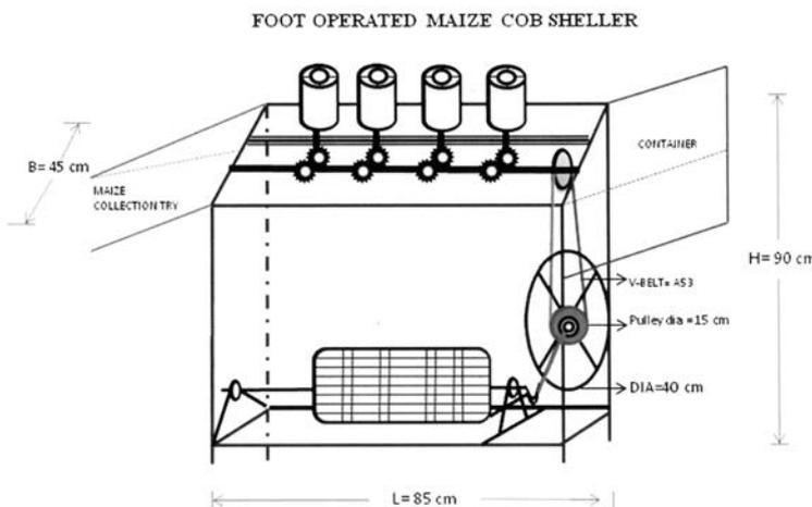
**Fig. 2** Isometric view of maize sheller used in shelling unit of designed prototype
