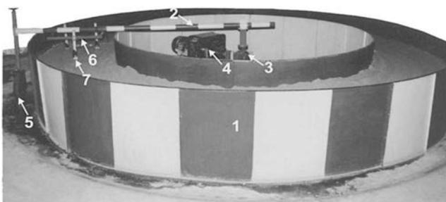
1. Soil bin 2. Horizontal beam 3. Worm gear unit 4. DC motor 5. Pneumatic wheel 6. Tool frame 7. Shovel
