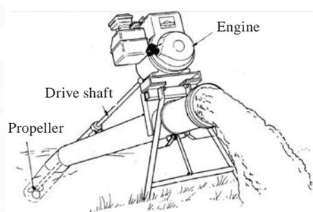
**Fig. 6** A giant-sized impeller mounted on drive shaft
