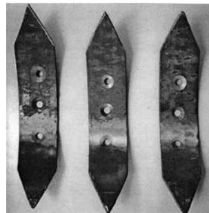
Fig. 3 Cumulative wear in shovels at different operating speed and time
