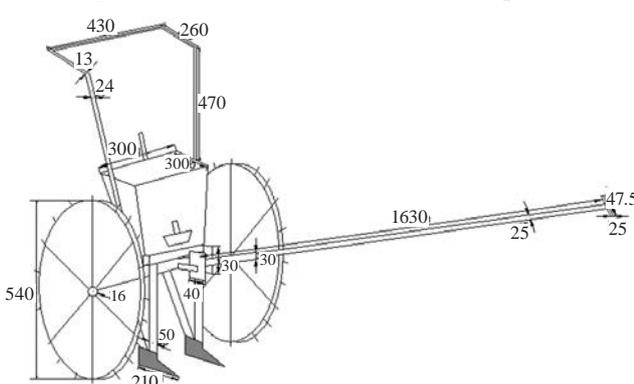
**Fig. 10** Vivek seed cum ferti drill (Self propelled operated)
