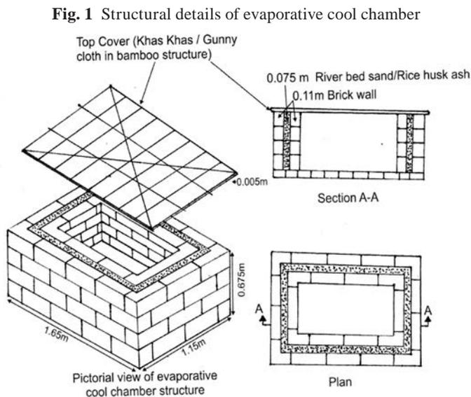
**Fig. 1** Structural details of evaporative cool chamber
