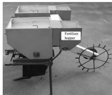
**Fig. 3** Two row subsoil organic mulch cum fertilizer applicator fitted with tractor
