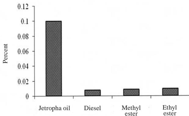
**Fig. 2** Kinematic viscosity of jatropa oil, diesel and their bio-diesels methyl ester and ethyl ester at 38 °C
