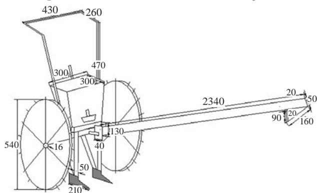
**Fig. 9** Vivek seed cum ferti drill (Manual operated)
