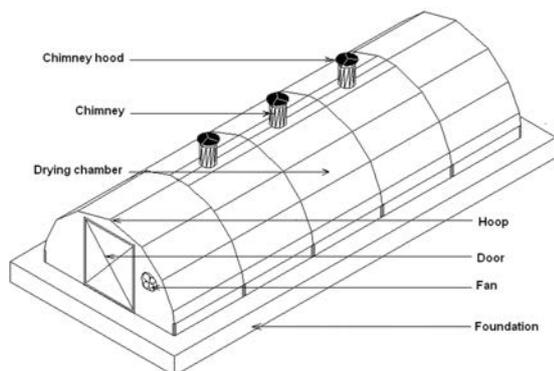
**Fig. 1b** Isometric view of solar tunnel dryer (100 kg/batch)
