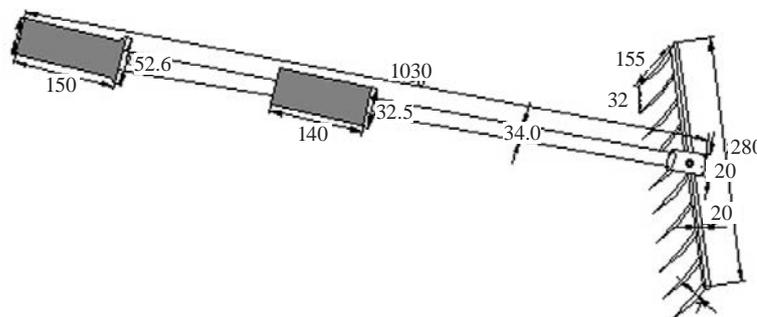
handle has been used. The width of coverage and spike spacing cannot be adjusted in traditional rakes. In the improved garden rake the handle has been made with MS pipe with two rubber grips (Fig. 2). The length and diameter of the handle and grip is 1,030 and 19 mm and 150 and 32.5 mm, respectively. The weight, field capacity and price of the improved garden rake are 1.25 kg, 83.3 m<sup>2</sup>/h and Rs.150 per unit, respectively.
