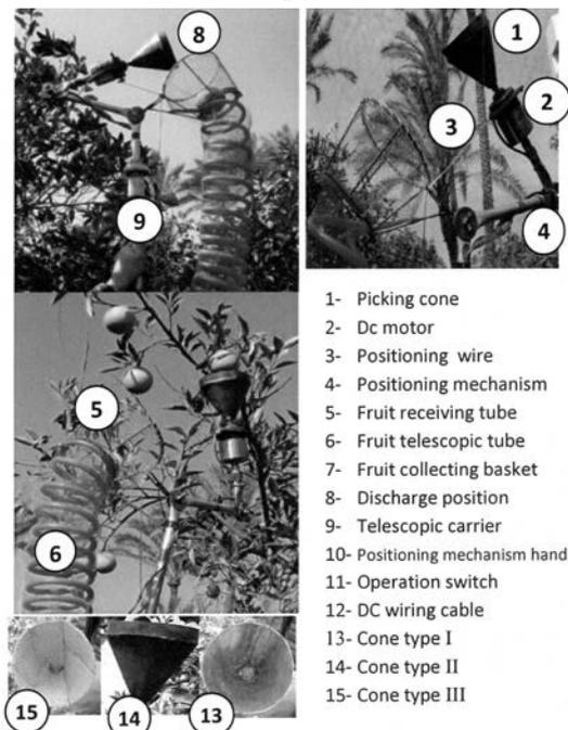
Fig. 2 Schematic diagram of rotary cone picking head
