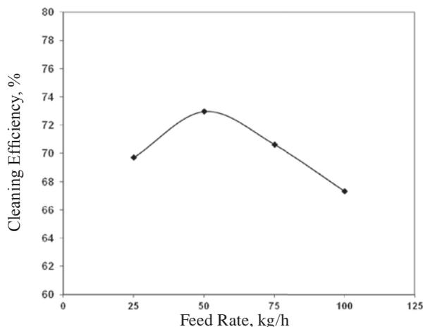
Fig. 3 Effect of Feed Rate on Cleaning Efficiency
