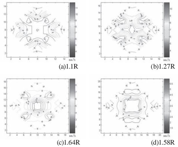
**Fig. 9** The square layout for cumulative water distribution of sprinkler type BPXH30
