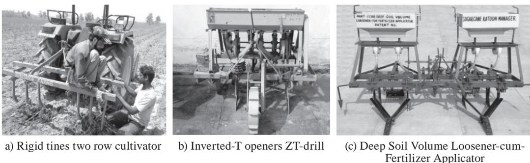
**Fig. 1** Different equipment used in the experiment
