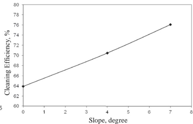
Fig. 6 Effect of Slope on Cleaning Efficiency
