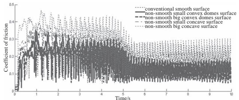
**Fig. 11** Frictional characteristic curves between the rape pod shell and various surface morphologies
