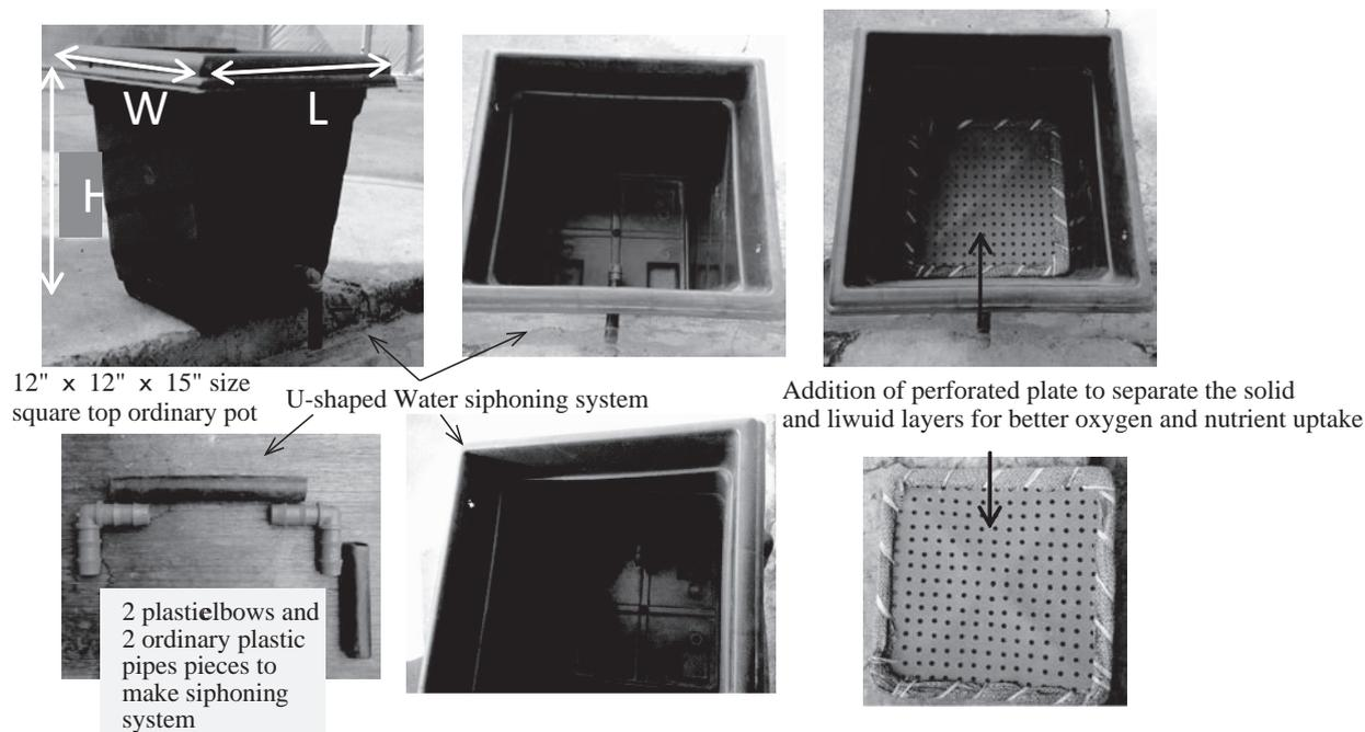
Fig. 2 Design details of pot, indigenously developed water siphoning system and perforated plate
