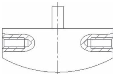
**Fig. 4** Schematic of ship-shaped collet of the upper frictional part
