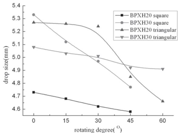
Fig. 7 Relationship between drop size and rotating degree
