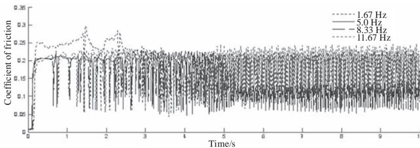
**Fig. 13** Frictional characteristic curves between the rape pod shell surface and the smooth surface at the various reciprocal frequencies
