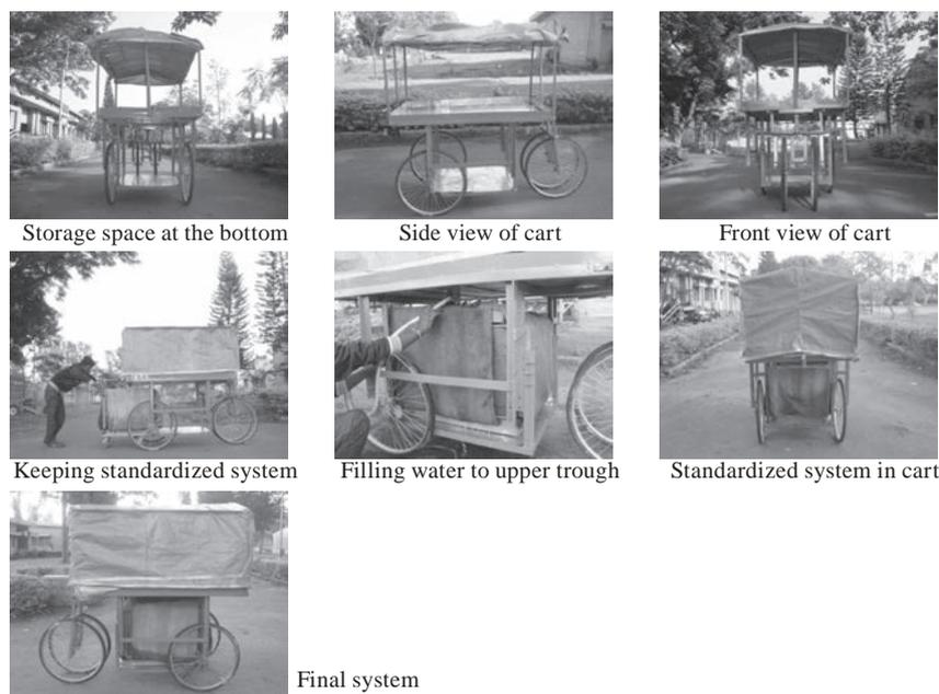
**Plate 1** Stepwise operation of modified pushcart
