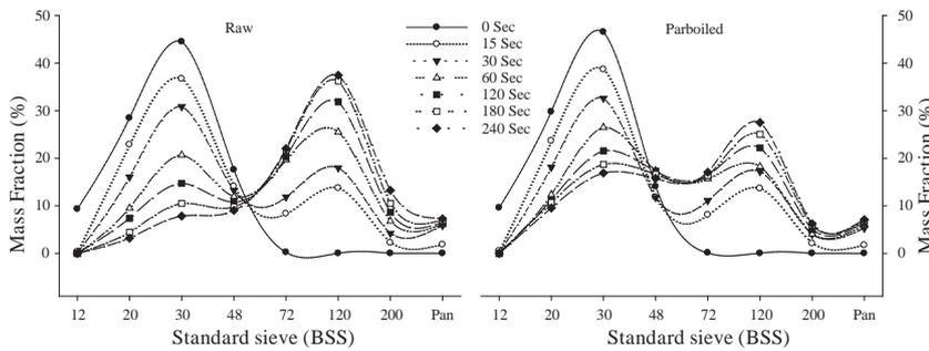
**Fig. 1** Process dependent particle size distribution kinetics of ground rice fractions
