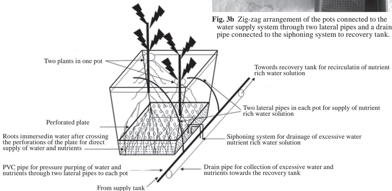
Fig. 3a Connection of the nutrient rich water supply system through the lateral pipes and siphoning system for drainage of the excessive water to the drain pipe connected to recovery tank.
