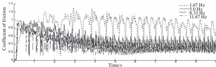
**Fig. 14** Frictional characteristic curves between the rape stalk and the bionic large convex dome surface at the various reciprocal frequencies
