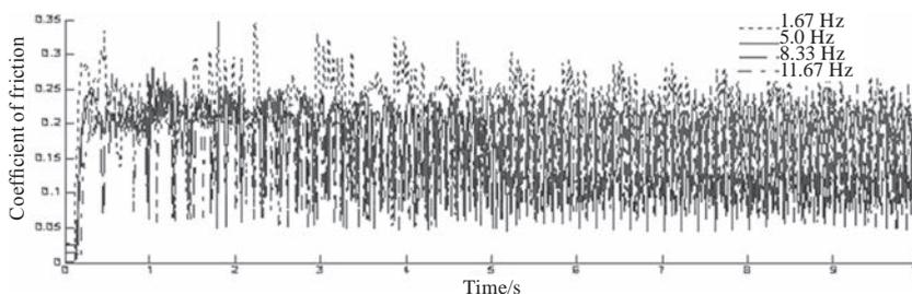
**Fig. 15** Frictional characteristic curves between the rape pod shell surface and the bionic large convex dome surface at the various reciprocal frequencies
