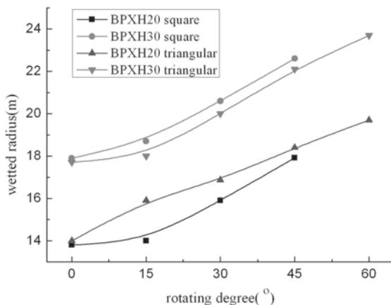
Fig. 6 Relationship between wetted radius and rotating degree
