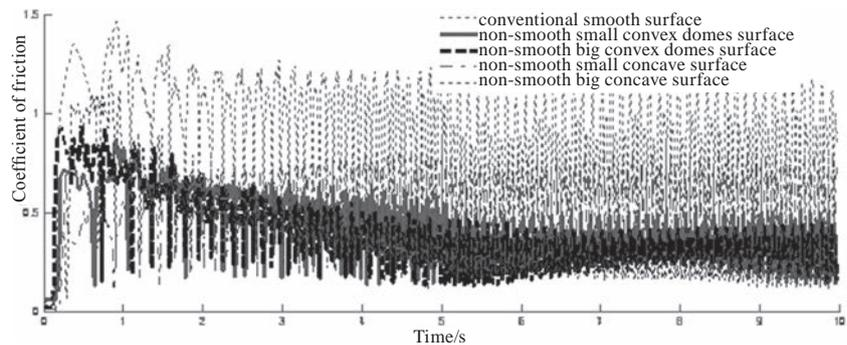
**Fig. 10** Frictional characteristic curves between the rape stalk and various surface morphologies
