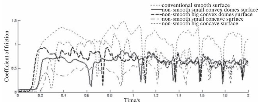
Fig. 18 The frictional characteristic curves between the rape stalk and various surficial morphology at the frequency of 8.33 Hz within 2 second
