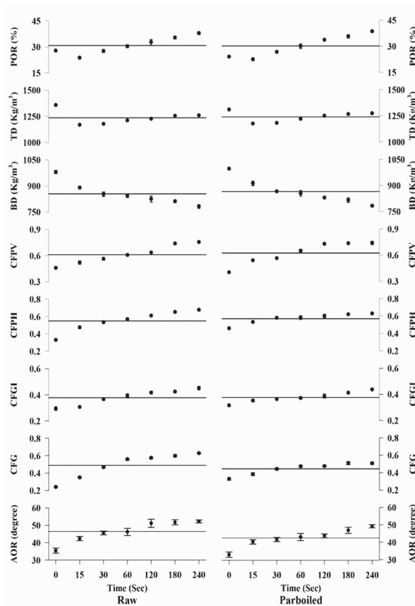
Fig. 4 Gravimetric and frictional characteristics of process and time dependent ground rice fractions
