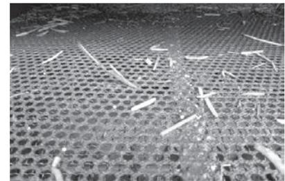
Fig. 17 The adhesion of the rapeseeds cleaning sieve with the non-smooth bionic surface
