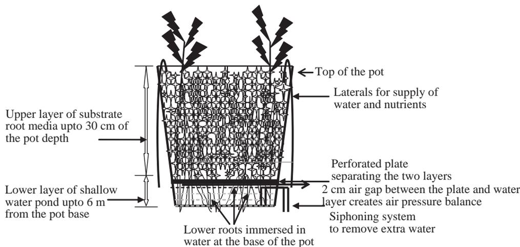
Fig. 1 Sectional view of the pot design of Hybrid Hydroponic Technology (HHT) having two layers; the upper layer of solid porous media and the lower layer of shallow water pond as separated by the perforated plate, and connected with water siphoning system.
