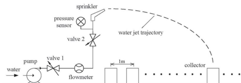
Fig. 2 The experiment system
