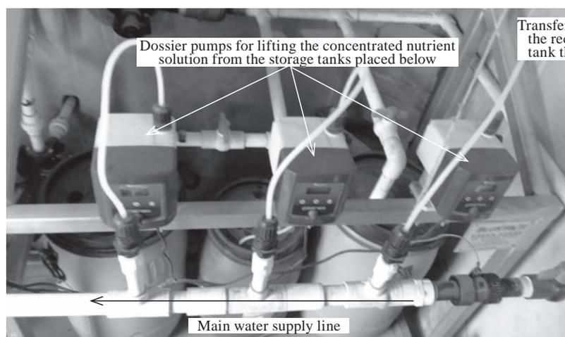
**Fig. 5** Indigenously developed nutrient dossier system for automatic mixing of nutrients to the main water line entering to the supply tank using three dossier pumps for Grow, Micro and Bloom part of nutrient components.
