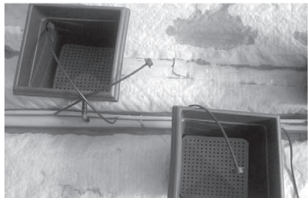
Fig. 3b Zig-zag arrangement of the pots connected to the water supply system through two lateral pipes and a drainage pipe connected to the siphoning system to recovery tank.
