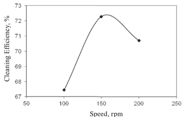
Fig. 4 Effect of Speed on Cleaning Efficiency
