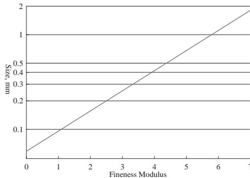
**Fig. 2** Relationship between the fineness modulus and average particle size
