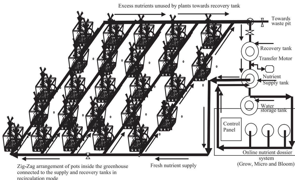
Fig. 4 Schematic view of the indigenously developed pot based hybrid hydroponics technology (HHT) with closed loop water and nutrient supply and recovery system (recirculation mode) coupled with online nutrient dossier system.
