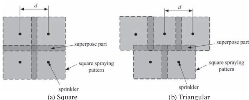
Fig. 3 Layout of the sprinklers in a square (a) and triangular pattern (b)
