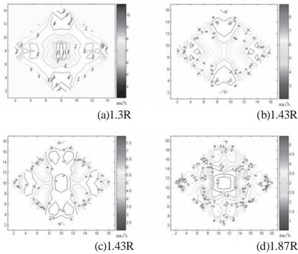
**Fig. 8** The square layout for cumulative water distribution of sprinkler type BPXH20
