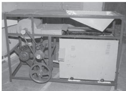
Fig. 2 Developed cumin cleaner cum grader
