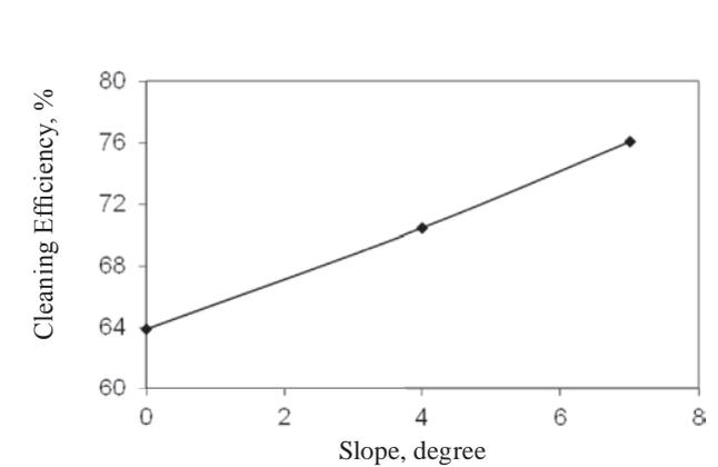
Fig. 8 Effect of Slope on Cleaning Efficiency
