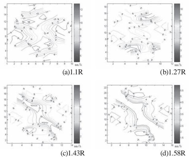
**Fig. 11** The triangular layout for cumulative water distribution of sprinkler type BPXH30
