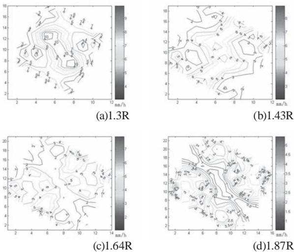
**Fig. 10** The triangular layout for cumulative water distribution of sprinkler type BPXH20
