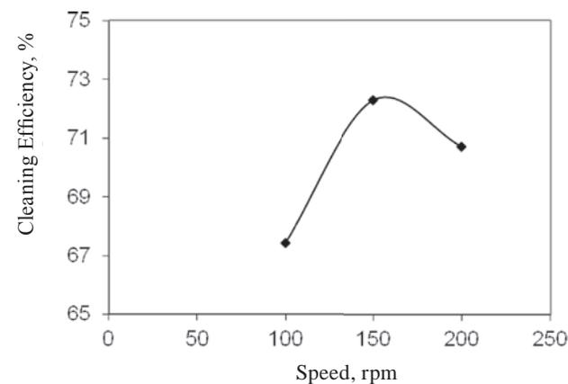
Fig. 7 Effect of Speed on Cleaning Efficiency
