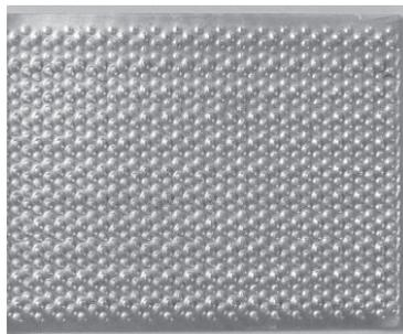
**Fig. 8** Non-smooth convex dome surface
