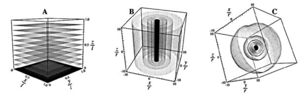
**Fig. 4** Three different diffusion bases of Fick's models used for the three geometrical shapes of Guavas (A) infinite plane model for plate slices shape; (B) finite cylinder model for cylindrical shape and (C) finite sphere model for spherical shape.
