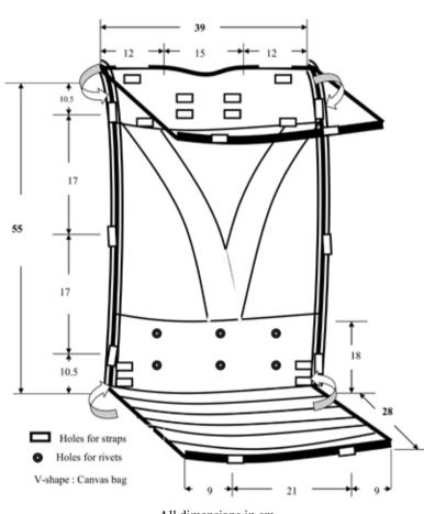
All dimensions in cm. Note: Arrows show the hinge points to fold the pack at its top and bottom Fig: Developed external frame backpack
