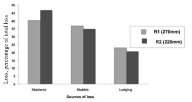
Fig. 9 Contribution of the various sources of loss to the total unrecovered grains in  $a \ 2 \times 5 \times 5$  factorial experiment.
