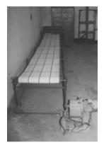
Fig. 1 Test rig for metering of seeds through sticky belt
