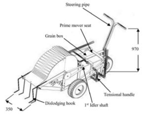
Fig.4a Isometric left side view of stripper harvester
