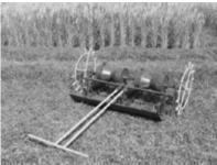
Fig.1 Four row manual drum seeder
