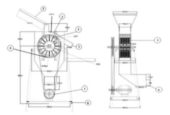
Side view Front View 1. Feed hopper, 2. Hulling cum deseeding unit, 3. Pegs, 4. Concave sieve, 5. Pulp outlet, 6. Hull outlet, 7. Motor, 8. Frame **Fig. 2** Tamarind Huller cum Deseeder
