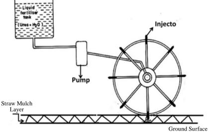
Fig. 1 Conceptual sketch of nitrogen (liquid urea) application mechanism
