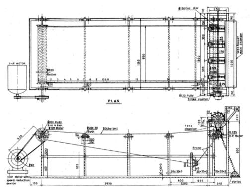
Fig. 2 Test rig for performance evaluation of cup feed metering device
