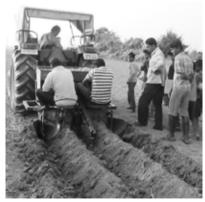
**Fig. 2** Performance evaluation of the 2-row semi-autimatic potato planter
