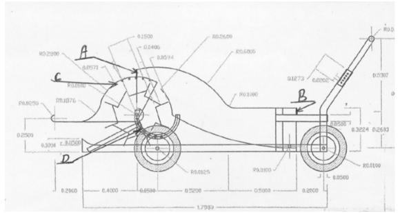
Fig. 2 Side view of stripper header.
