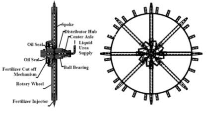
Fig. 6 Views of Nitrogen (liquid urea) metering and cut-off mechanism
