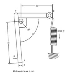
Fig. 4 Crank Lever for cut-off mechanism
