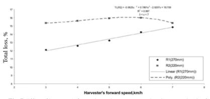
Fig. 7 Effect of harverter's forward speed on unrecovered grains at two levels of rotor height
