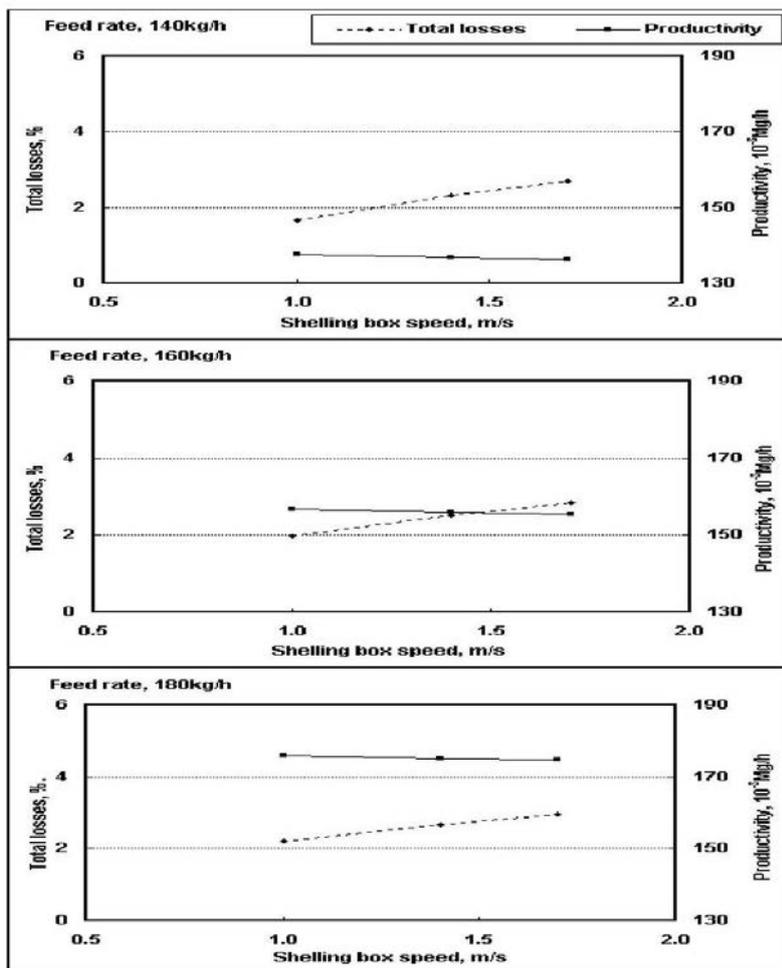
**Fig. 5** Effect of feeding rate on damaged, unshelled seeds and total losses for the sheller before and after modification at pods moisture content about 17.12 % w.b. and shelling box speed of 1.4 m/s
