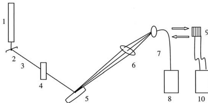
1: Laser source; 2: Mirror; 3: Laser beam; 4: Filter; 4: Filter; 5: Sample; 6: Convex lens; 7: Detector; 8: Lux meter; 9: Photovoltaic cell; 10: Avo meter.
