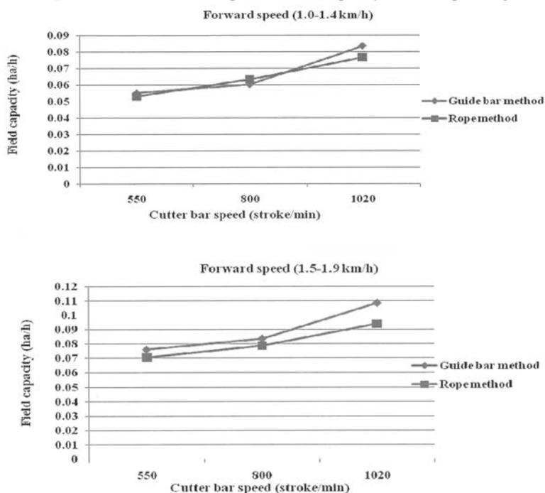
**Fig. 10** Effect of method of collection on field capacity in trench planting
