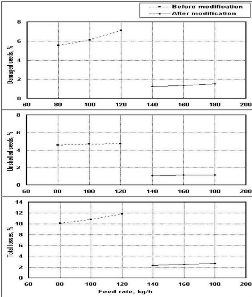
**Fig. 6** Effect of feeding rate on shelling efficiency at pods moisture content about 17.12 % w.b. and shelling box speed of 1.4 m/s
