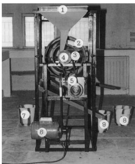
1. Feed hopper, 2. Outer screen, 3. Inner screen, 4. Main shaft, 5. Gear box, 6. Motor, 7. Cleaned seed outlet, 8. Partially cleaned seed outlet, 9. Impurities outlet
