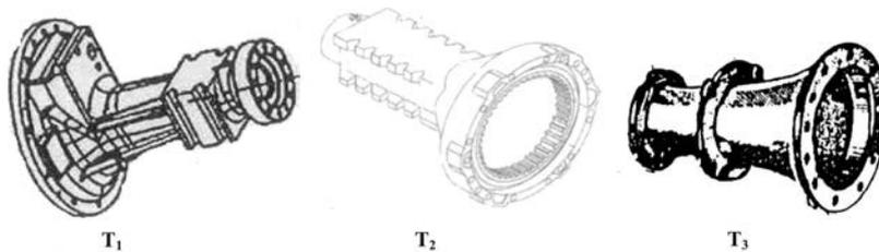
**Fig. 3** Fitment technique of different safety frame on axle housing
