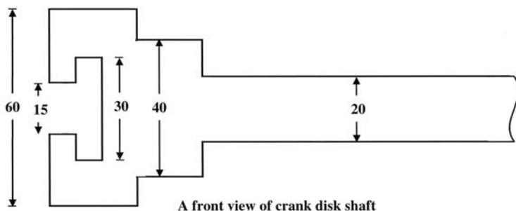
A front view of crank disk shaft
