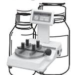
Table top, manual load, digital torque meter ideal for cap testing. **TME2**
