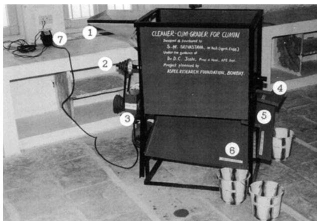
1. Feed hopper, 2. Main shaft, 3. Gear box, 4. Cleaned seed outlet, 5. Partially cleaned seed outlet, 6. Impurities outlet, 7. Energy meter
