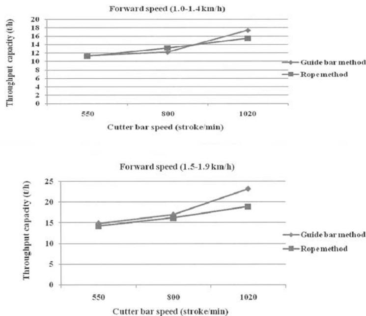
**Fig. 13** Effect of method of collection on material capacity in trench planting
