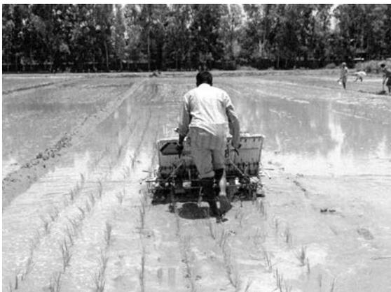
**Fig. 3** A view of self propelled 4-wheel type paddy transplanter in operation
