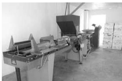
Fig. 17 High-tech greenhouse machinery; (Right) vacuum seeder and (Left) produce washing, waxing, grading and sorting machine
