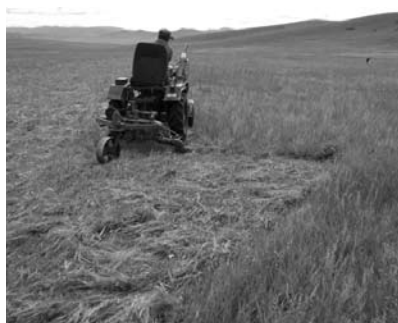
Fig. 2 Testing process of tractor BJ-200 (China) for hay cutting
