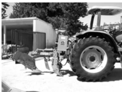
Fig. 5 Laser guided special plow (Delfino 3s) attached to specially equipped sizable tractor (This photo was provided by Issa Gammoh, Associate Professor at the Faculty of Agriculture, University of Jordan, Amman, Jordan).
