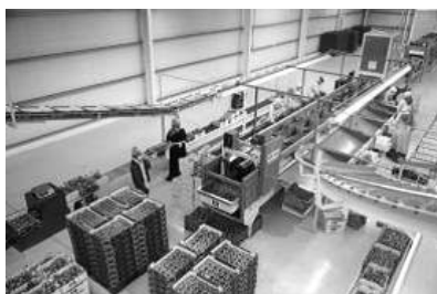
Fig. 17 High-tech greenhouse machinery; (Right) vacuum seeder and (Left) produce washing, waxing, grading and sorting machine
