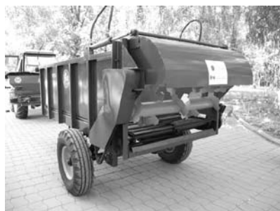
Fig. 5 The compost windrow-forming car (Developed by KNAU and JICA)
