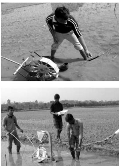
**Fig. 1** Measurement of pushing force using spring balance
