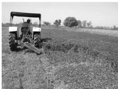
**Fig. 1** Tractor operated cutter bar type fodder harvester
