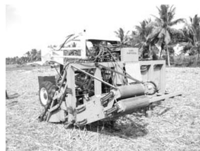
**Plate 2** Isometric view of tractor operated whole cane combine harvester
