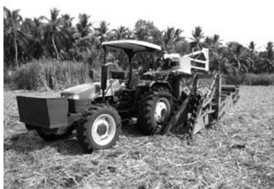
**Plate 1** Front view of tractor operated whole cane combine harvester
