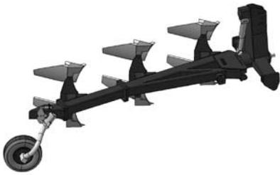
**Fig. 1** Schematic view of the primary design of moldboard plow used in the research
