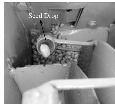
**Fig. 7** Close view of precision seed metering mechanism
