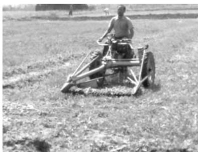
**Fig. 2** Engine operated riding type fodder harvester
