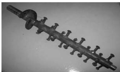
**Fig. 1** Rotor shaft with auger and stud assembly
