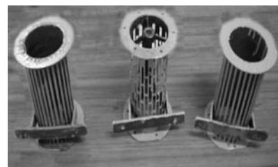
Fig. 4 Cylindrical sieves made up of square bars, sheet having oblong hole and cylindrical rods
