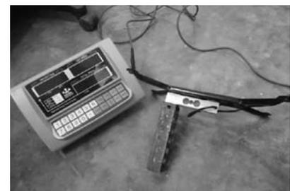
**Fig. 15** Developed dynamometer
