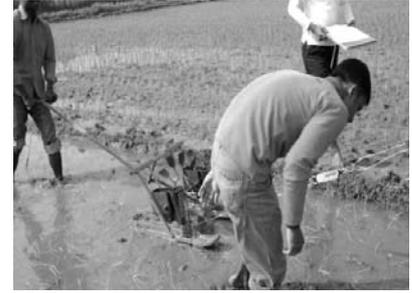
**Fig. 10** Force measurement in the field by spring balance in traditional method
