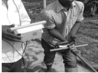
**Fig. 9** Force measurement in the field by dynamometer
