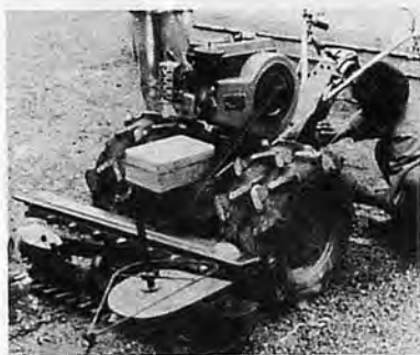
Fig.6. Side-delivery paddy harvester in Kiangsu province.
