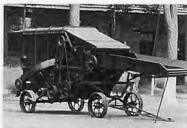
Fig.3. A conventional wheat thresher manufactured by the Red Star Commune near Peking.
