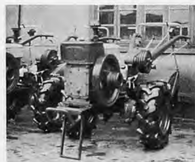
Fig.2. A Chinese power tiller—Model Tung Fung-12, produced in Kiangsu province.
