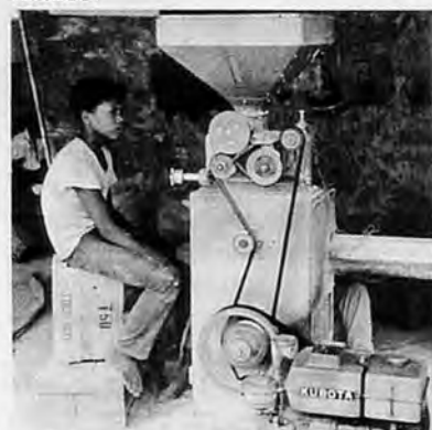
Fig.3. An example of advanced husking-whitening unit to be used by small rice mills. (Capacity: 200kg/h on paddy in above photo, capacity: 500kg/h on paddy in below photo.)
