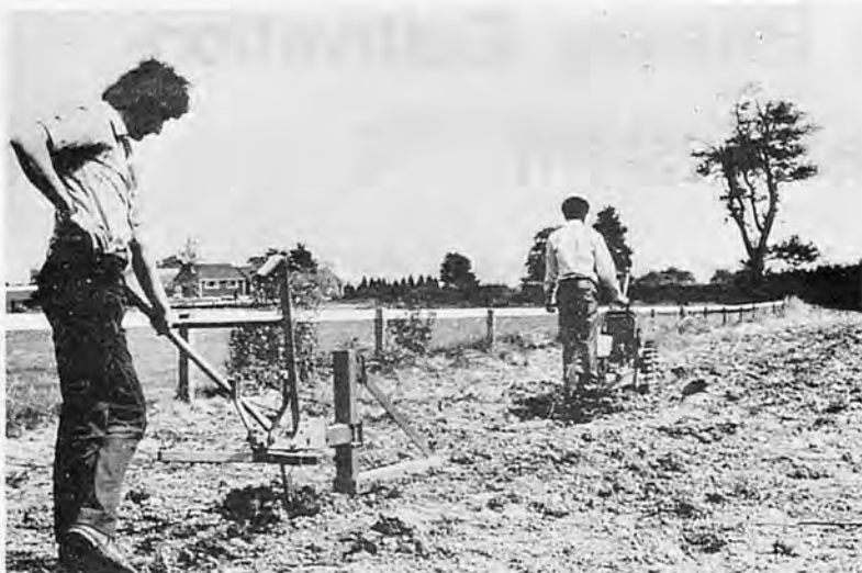
Fig.1. The plough remains stationary while the power unit drives off to the limit of the cable's length.
