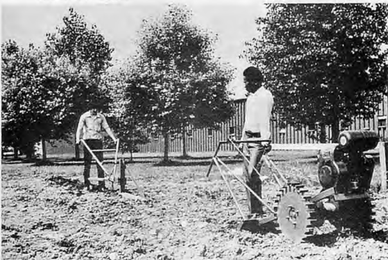
Fig.2. The power unit is now stationary and draws the plough towards itself by means of the cable and winch.
