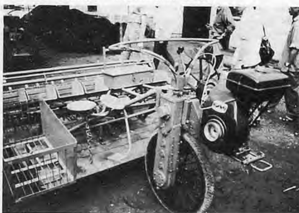
Fig.5. Riding type power operated Chinese transplanter developed in Shanghai.
