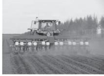
Fig. 3(a) Precision Variable Rate Fertilization Seeder
