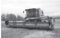
Fig. 6 Large Intelligent Grain Combine Harvester with 10 kg/s Feed Rate
