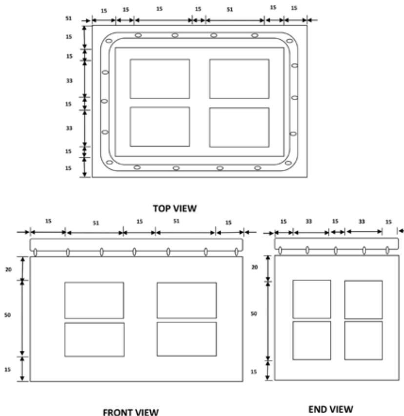
**Fig 1** Dimensions of evaporative cooling storage
