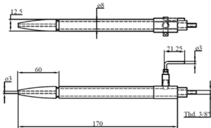
**Fig. 3** View of spoke with injector
