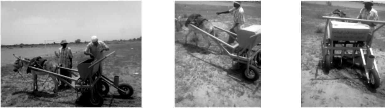
Fig. 2 Groundnut planting machine in operation
