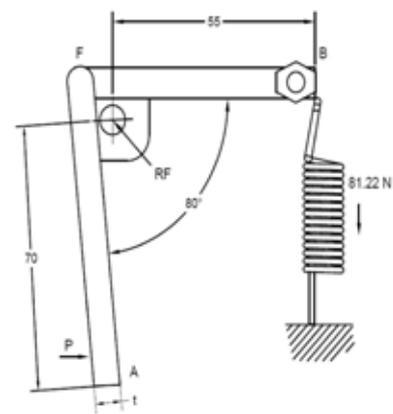
**Fig. 4** Crank Lever for cut-off mechanism
