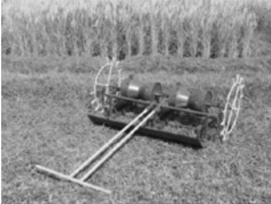
**Fig.1** Four row manual drum seeder
