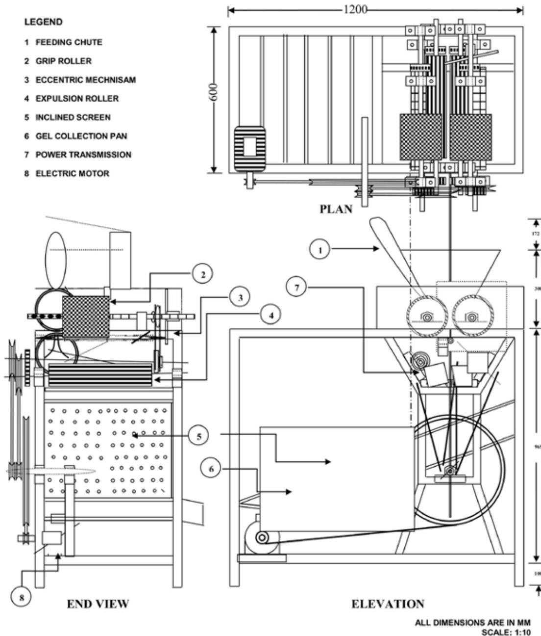
Schematic diagram of developed aloe vera gel expulsion machine
