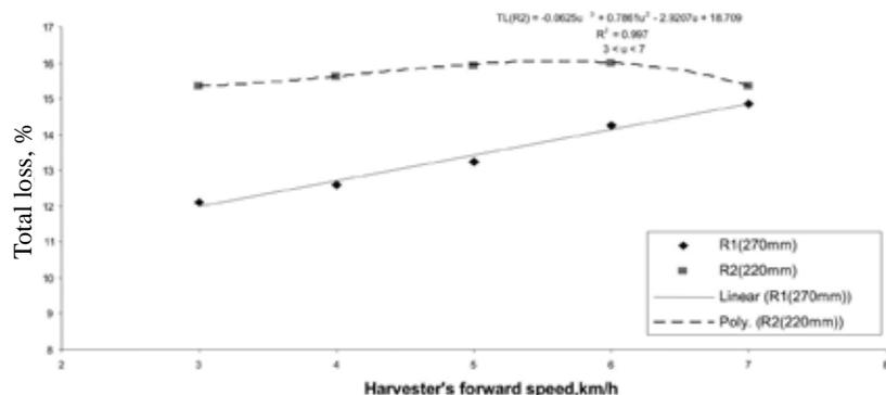
**Fig. 7** Effect of harvester's forward speed on unrecovered grains at two levels of rotor height
