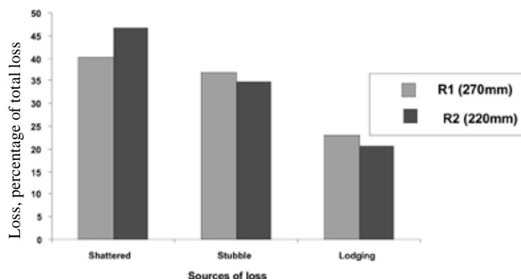
**Fig. 9** Contribution of the various sources of loss to the total unrecovered grains in a  $2 \times 5 \times 5$  factorial experiment.
