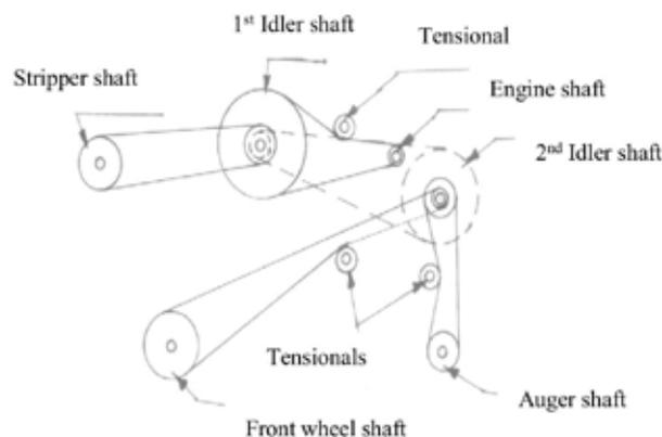
**Fig. 4b** Machine power transmission layout
