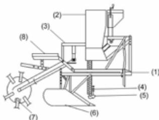
1- Main frame; 2- Seed Box; 3-Seed plate; 4- Seed tube; 5-Furrow opener; 6- Ridger; 7- Ground wheel; 8- Seat for potato dropper
