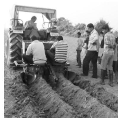
**Fig. 2** Performance evaluation of the 2-row semi-automatic potato planter
