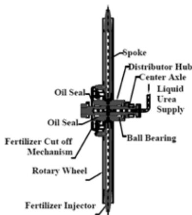
Fig. 6 Views of Nitrogen (liquid urea) metering and cut-off mechanism
