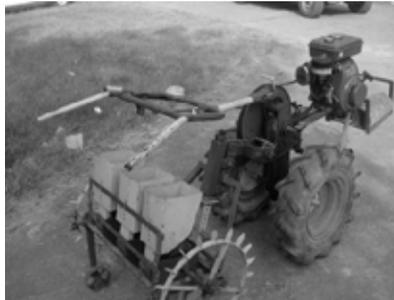
**Fig.5** Self propelled hill seeder
