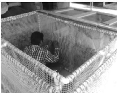
b. Placement of coconut chips in annular space
