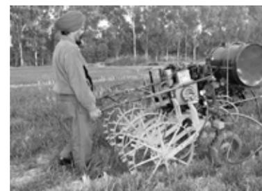
**Fig. 8** View of developed nitrogen (liquid Urea) Applicator operation under actual field conditions
