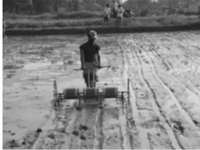
**Fig.2** Six row manual drum seeder
