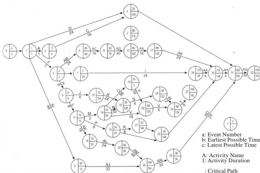
The expected completion time of overhauling was 192 hours. The total variance of completion time was 8 hours. The largest variance was associated with activity AM viz., piston liners inserting, reboring, crankshaft balance and crack checking. The analysis revealed the probability of completing the overhauling ranged from 0.299 to 0.331 for completion duration of 185 to 200 hours.
