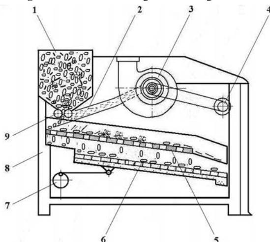
**Fig. 2** Small-sized grain cleaning machine
