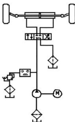
**Fig. 7** Schematic diagram of the steering circuit
