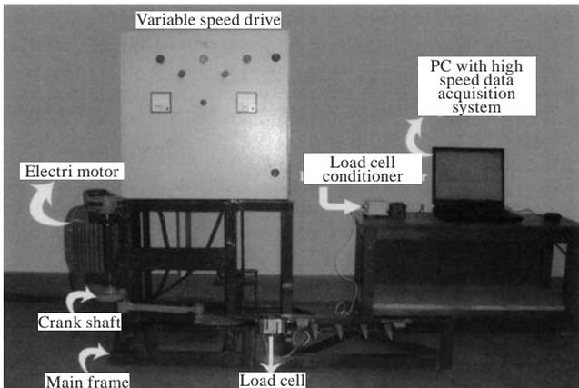
Fig. 2 Load cell connected to wearing plate of cutter bar
