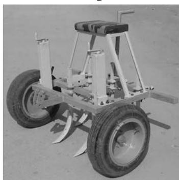
**Fig. 2** Pneumatic wheeled MPT frame with seeding attachment
