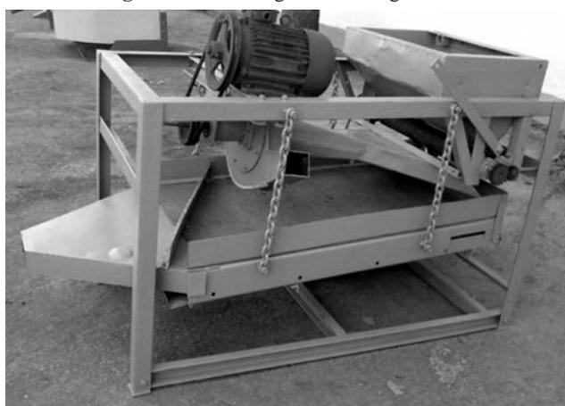
completeness of the heaps mastication were up to standard of an initial request, and admissible damage of grain is at a frequency of roller rotation of 800...1,000 rpm.
