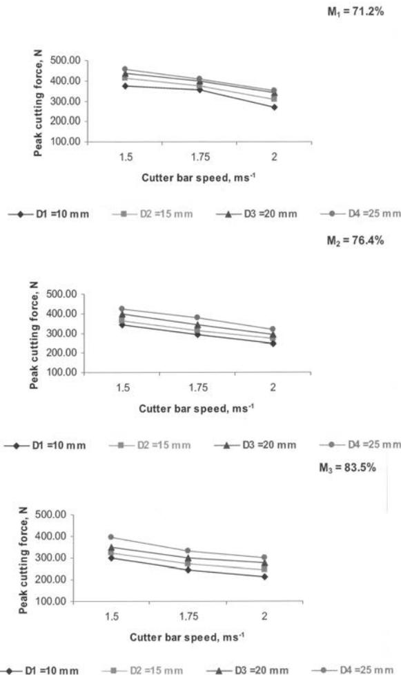
**Fig. 6** Effect of cutter bar speed on peak cutting force at selected levels of diameter and moisture content of maize stalk for 90.0 mm stroke length of cutter bar ( $L_2$ )
