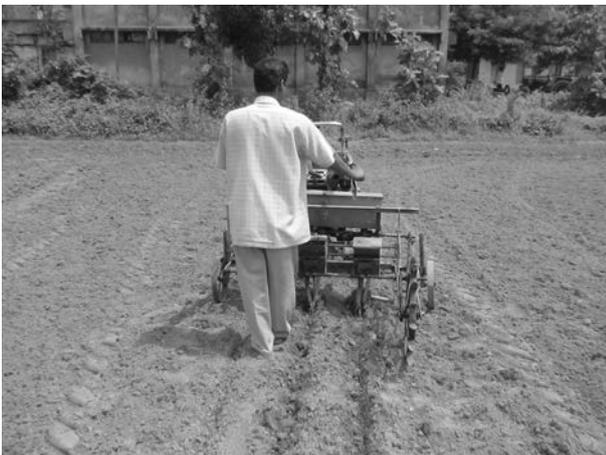
**Fig. 4** Field evaluation of the power tiller operated planter (side view)
