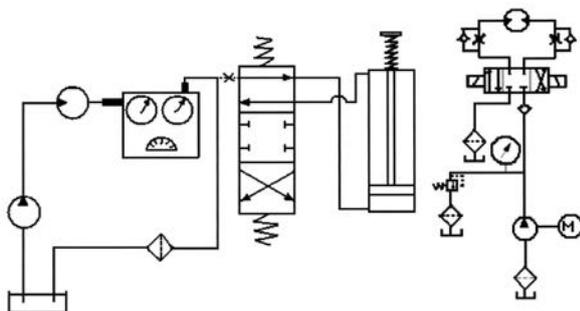
**Fig. 4** Setup for testing the hydraulic cylinder and schematic circuit
