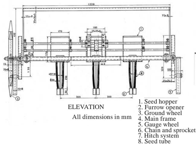
**Fig. 2** Schematic diagram of power tiller operated planter (side view)
