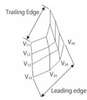
**Fig. 2** Control points of developed blade at zero degree orientation in single patch (GS methods)
