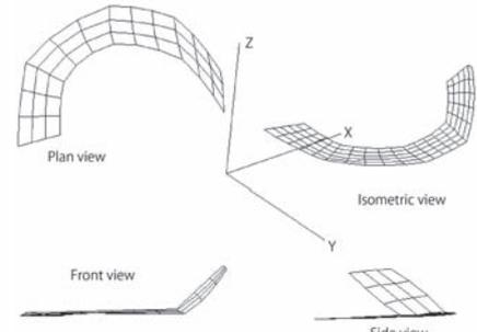
**Fig. 5c** Three-dimensional surface developed for Japanese C-type blade
