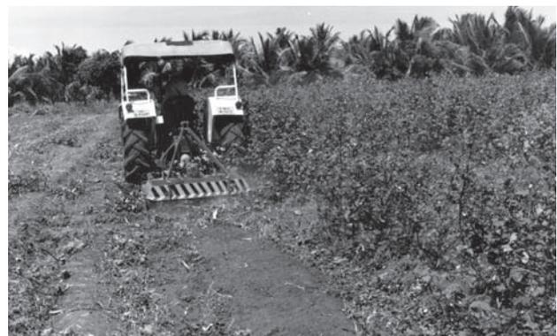
**Fig. 1** Tractor operated roto slasher
