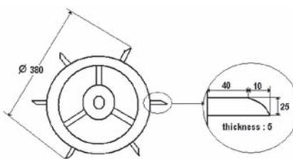
Fig. 3 A view of the lama (flat)-tooth beater
