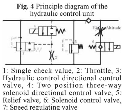
**Fig. 3** Block diagram of the hydraulic controller
