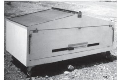
Fig. 6 Photograph of small scale production dryer (open)
