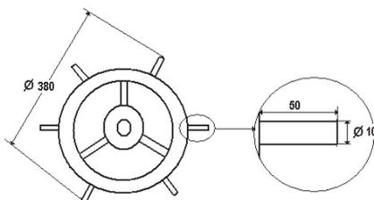
Fig. 2 Dimensions of the spike-tooth beater (all measurements are mm)
