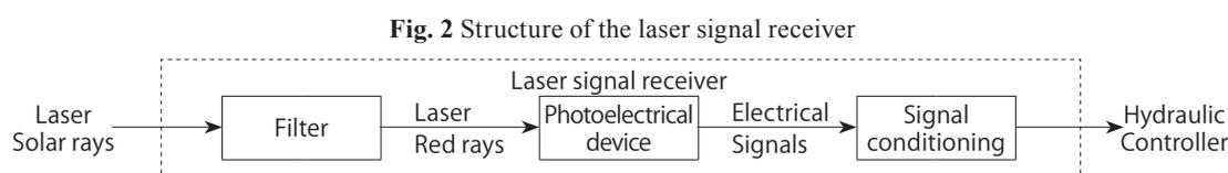
with the intensive disturbance of solar rays and the processing of low-power electrical signals transduced by photoelectrical device. The structure of the laser signal receiver is shown in Fig. 2.
