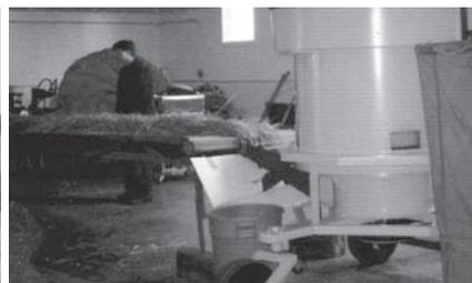
**Fig. 2** VC2A vertical axial-flow threshing unit made in Prairie Agricultural Machinery Institute, Canada
