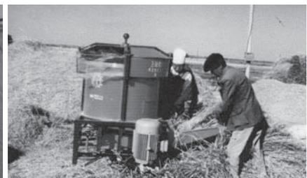
**Fig. 3** VT1.0 vertical thresher worked in the field
