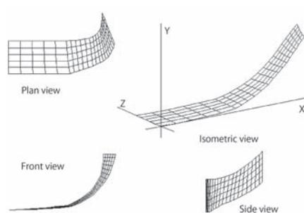
**Fig. 5a** Three-dimensional surface developed for C-type blade
