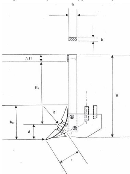
**Fig. 2** Development of inverted - T type furrow opener
