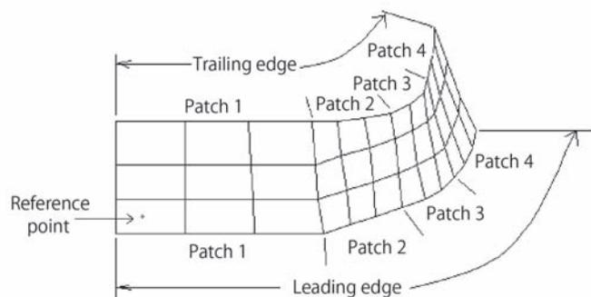
**Fig. 4** The complete blade surface generated by joining four patches of control points
