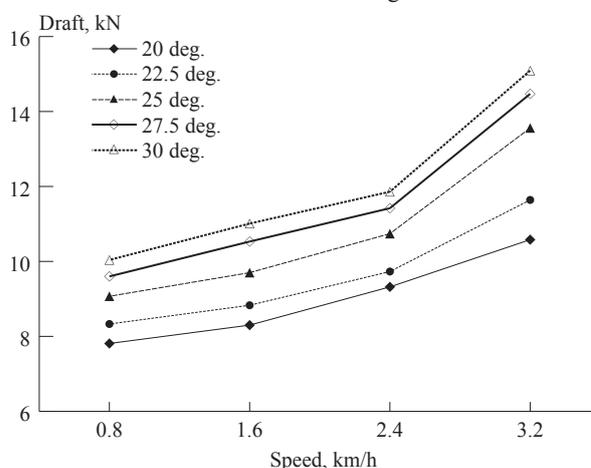
Ferguson tractors. The auxiliary tractor was used to pull the harvester - mounted tractor through the dynamometer with the harvester set at determined operating conditions and neutral gear position. Readings were taken at approximately every 30 m, along each row of ridge as the harvester moved through the test area. After this reading, the harvester was lifted out of the ground and the reading taken. The difference gave the draft of implement under that operating condition.
