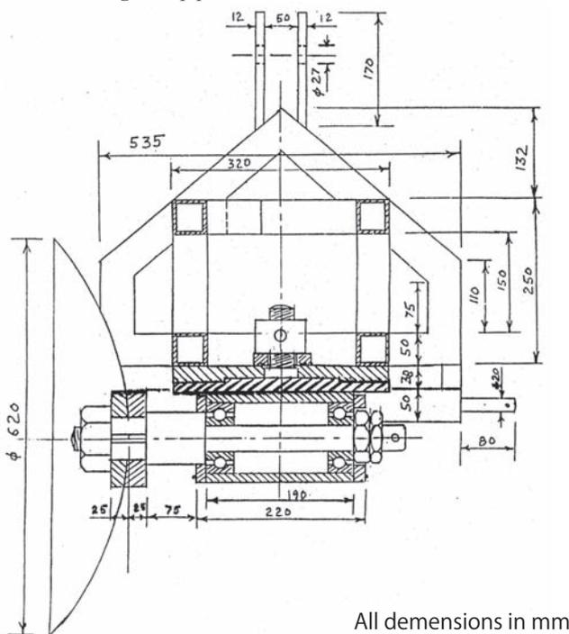
Fig. 2 Changing of disc - an easy process
