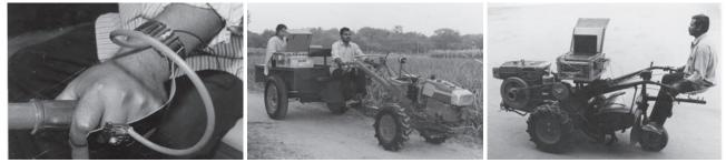
1998 and Ragni, et al., 1999) and fixed on the grip by tape (**Fig. 1**). The transducer was inserted between the middle and index fingers of left hand of each subject since the force output from index and middle finger is larger than that from ring and little finger (Fransson and Winkel, 1991). The right hand was used for operating the controls.
