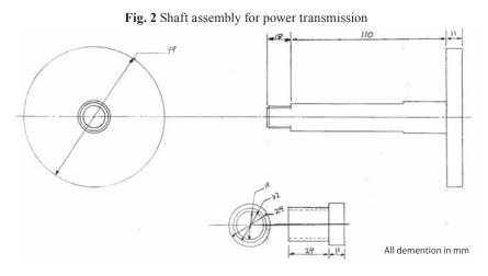
Plate 4 The modified universal joint Plate 5 Shaft assembly for power transmission
