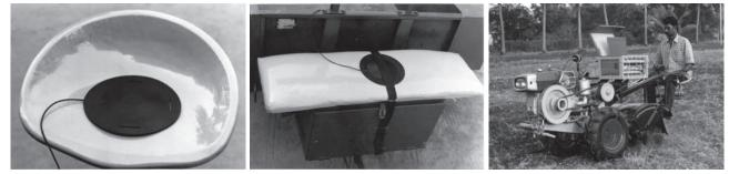
tion and noise analysis type 7700. On this base, pulse software such as data recorder type 7701 was installed. The entire system consisted of a portable data acquisition unitfront end type 2827, vibration and noise analysis software type 7700, data recorder type 7701 and triaxial seat accelerometer type 4322.
