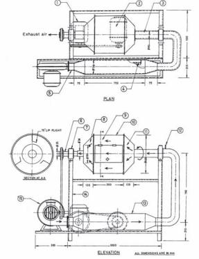
Reduction gear box, 2. Motor, 3. Hollow shaft, 4. Heating coil,
