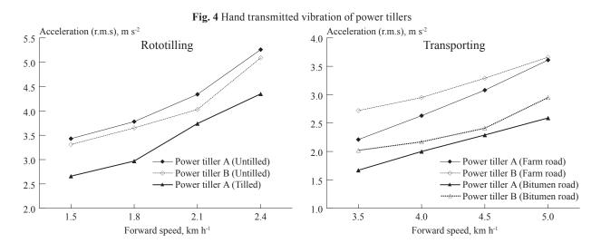
the prevalence of vibration induced white finger (VWF) and numbness of the hands will start very earlier. Hence, in order to increase the exposure time, the HTV of test power tillers need to be reduced. The vibration at the handle can be reduced by providing vibration isolators.
