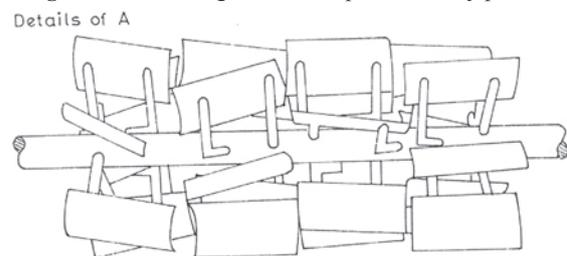
1. Six rectangular concave blades in one row, 2. Blade width 15 cm, 3. Blade depth 85 cm, 4. Blade angle w.r.t. shaft 30°
