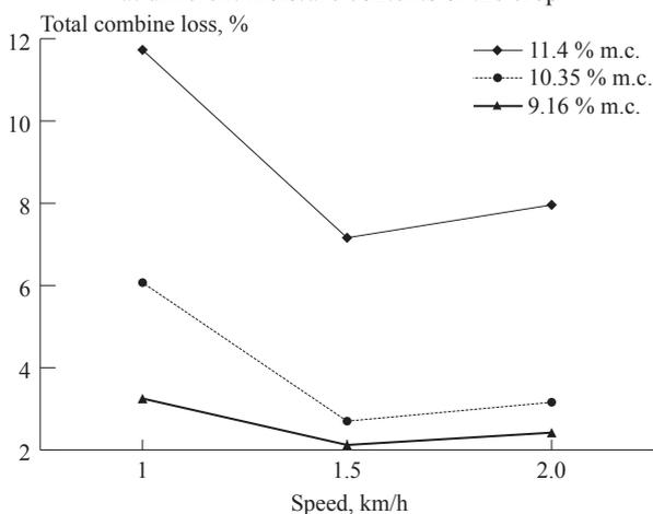
**Fig. 7** Effect of plot combine speed on grain breakage at different moisture contents of the crop
