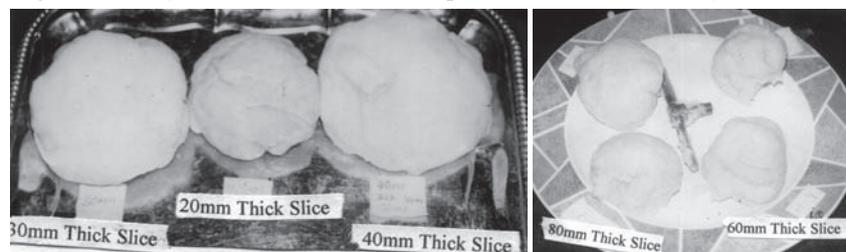
the first few rotations of the hammer remain stuck to the bottom of the pounding unit while the rest of the yam slices remain at the top, unbroken. It was also noticed that the size of the lumps of unbroken yam pieces increased with the size of the yam slice used for pounding.
