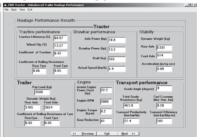
(TP), transport efficiency (TPE), fuel economy (FE) and upward grade resistance (GR) as described by Wong (1993). Fuel consumption of a tractor was calculated using the ASAE Standards (2001).
