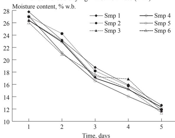
midity (humidity ratio) of drying air as well as the amounts of moisture removed at the three drying settings using the wet and dry bulb temperatures. The major aspect investigated was the ability of the dryer to reduce the material moisture from experimental conditions.
