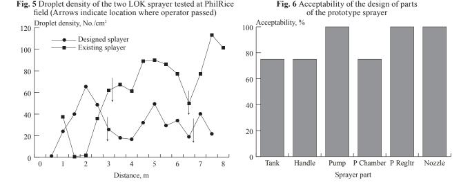
low as compared to that of the existing sprayer. Like the existing sprayer, however, it satisfied the minimum requirement of 20 droplets/ cm<sup>2</sup>. The effect of overlapping spray coverage during each pass was more obvious with the farmers' sprayer than with the designed sprayer. This was manifested by the rise in droplet density between operator paths. A more uniform coverage was seen when the droplet density remaind the same at any location relative to the path of the operator.
