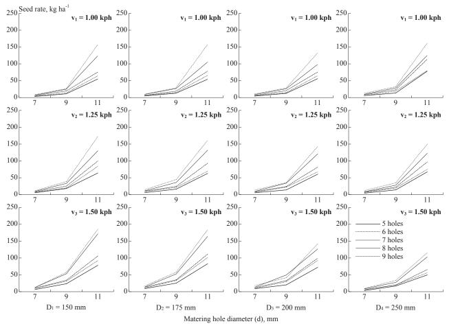
Fig. 4 Effect of hole diameter on seed rate at selected forward speed of operation for cylindrical drum (S1)
