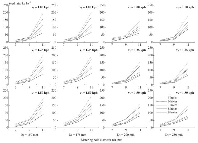
Fig. 5 Effect of hole diameter on seed rate at selected forward speed of operation for hyperboloid seed drum  $(S_2)$
