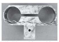
Fig. 4 The extended octagonal ring transducer fabricated based on simulation
