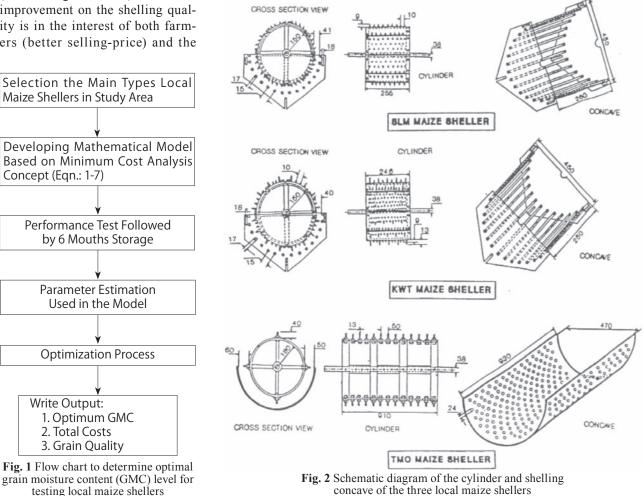
Fig. 1 Flow chart to determine optimal grain moisture content (GMC) level for testing local maize shellers
