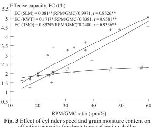
effective capacity for three types of maize sheller (+ SLM, \* KWT and # TMO)
