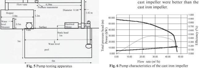
The differences of the total head, flow rate and overall efficiency between these two pumps were 0.46 m, 7.50 m<sup>3</sup>/h and 8.4 %, respectively. Power requirement of the pump with the brass cast impeller was 1 % higher than that of the pump with cast iron impeller and the flow rate was higher.
