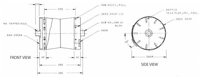
Fig. 3 Hyperboloid seed drum with baffle arrangement
