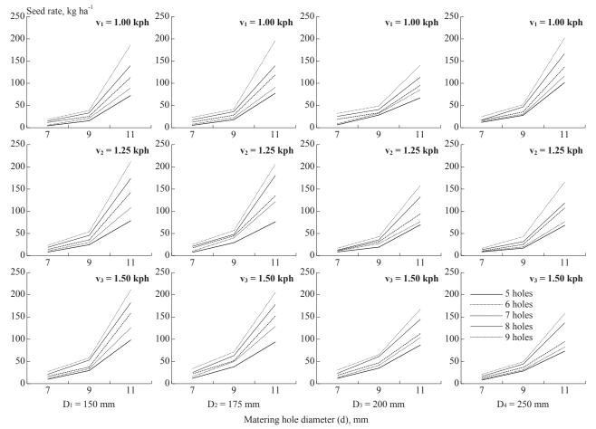
Fig. 6 Effect of hole diameter on seed rate at selected forward speed of operation for cylindrical ellipsoid drum (S<sub>3</sub>)
