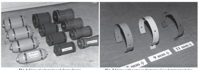
Fig. 1 View of selected seed drum shapes (150, 175, 200 and 250 mm diameter)
