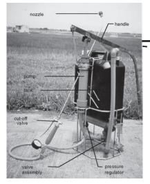
Fig. 3 The prototype's pressure regulator
