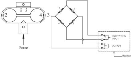
Fig. 5 Transducer and circuit diagram for measurement of forces
