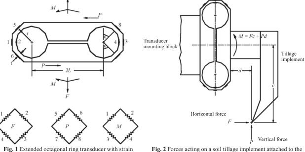
Fig. 1 Extended octagonal ring transducer with strain gauges for measurement of forces and moments
