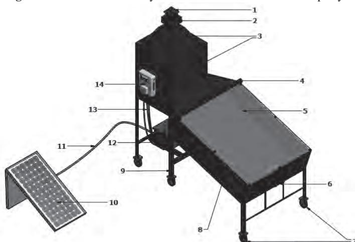
1. Chimney, 2. Outlet/exhaust fan housing, 3. Drying chamber hood, 4. Heating chamber, 5. Plain glass, 6. Inlet sensor fan, 7. Rollers, 8. Solar collector, 9. Angle iron support, 10. Solar panel, 11. Solar panel cable, 12. Inverter/battery unit, 13. Control unit cable, 14. Control unit
