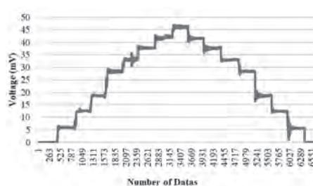
**Fig. 10** Cycles of loading and unloading of the OAE transducer during calibration with different weights for the horizontal force
