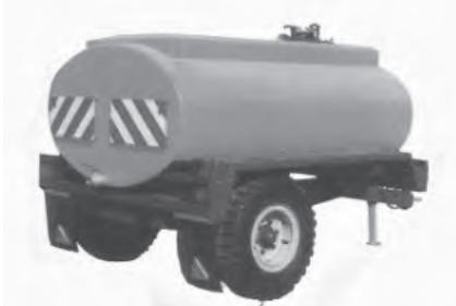
**Fig. 11** Trailed water transporting tank
