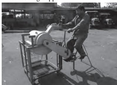
operated arecanut dehusker is shown in **Plate 2**. The details about dehusking cylinder and concave are given in **Fig. 2** and **Fig. 3**.
