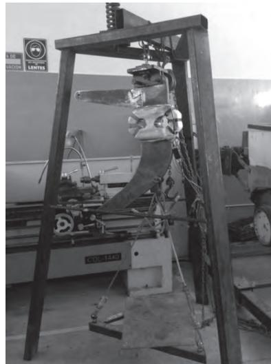
**Fig. 6** Calibration of torque transducer
