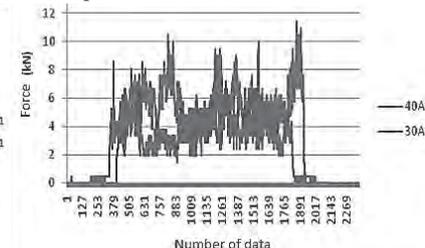
**Fig. 17** Graph showing the applied torque for the oscillating amplitude of 0.070 m and a working depth of 0.40 m
