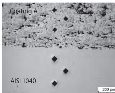
**Fig. 7** SEM overviews (back scattered electrons) of the polished cross-sections of the coating A and blade material
