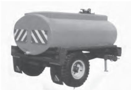
**Fig. 11** Trailed water transporting tank
