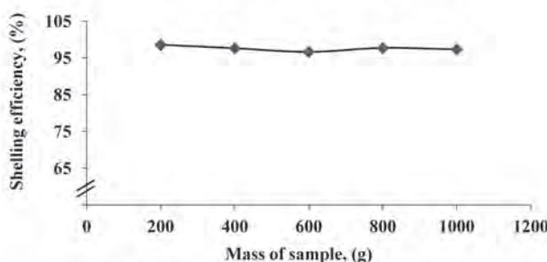
**Fig. 6** Effect of sample mass on shelling efficiency at speed of 200 rpm and clearance of 10 mm
