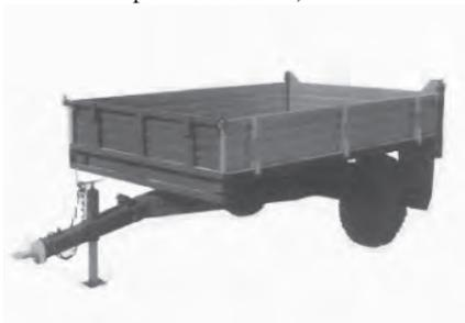
**Fig. 8** Four-ton trailer transport trailer (equipped with braking system, lighting and dumper mechanism)
