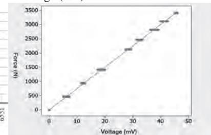
**Fig. 11** Shows the Linearity of calibration of horizontal force. The obtained equation was: Force (N) = 21.97 + 47.74 Voltage (mV)
