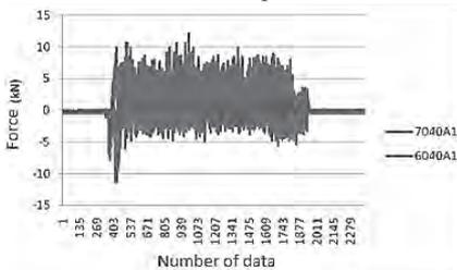
**Fig. 16** Comparative force demand at rigid tine and vibration (amplitude of 0.070 m) to the same depth of 0.40 m and speed of 1.5 km h<sup>-1</sup>. Graph (7040A1) shows the draft force for vibrating tine working at 0.40 m depth. Graph (40A1) shows the draft force for rigid tine working at 0.40 m depth
