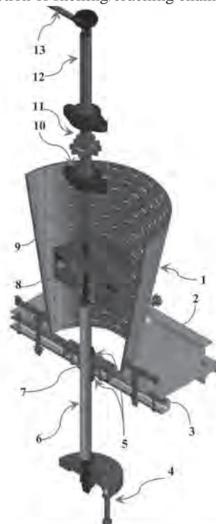
1. Fixed part, 2. Base of shelling chamber, 3. Screw for balance, 4. Handle, 5. Two nuts to tie screw, 6. Screw rod, 7. Fixed nut, 8. Rotary part, 9. Protrusion, 10. Pillow block bearing, 11. Sprocket wheel, 12. Rotational shaft, 13. Pointer
