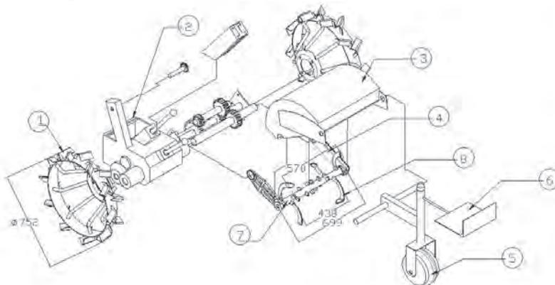
1. Cage wheel, 2. Gear Box, 3. Mud cover, 4. Power transmission chain, 5. Depth control cum *Biasi* wheel, 6. Operator seat, 7. Shaft, 8. C- type tines
