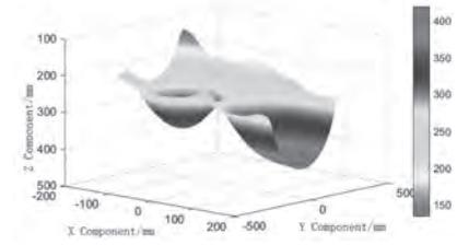
A and B are limited to  $\pm 80^\circ$  and the driven angle of chain C is limited to  $\pm 90^\circ$ . Then the lowest accessible boundary and the highest accessible boundary are achieved by MATLAB shown in **Fig. 2** and **Fig. 3**.
