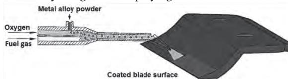
material codes “B” powder alloys by thermal spraying application (12 blades were coated).
