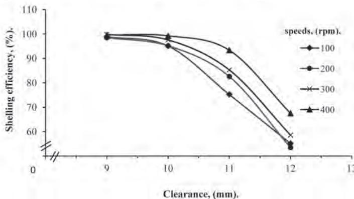
**Fig. 5** Effect of the tested clearance on the shelling efficiency at different speeds
