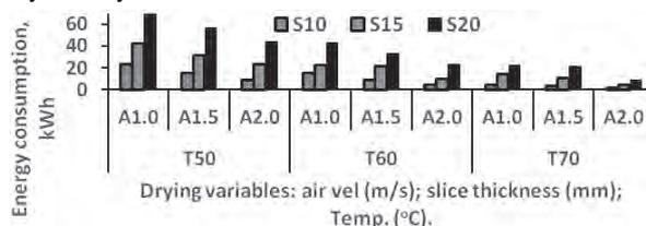
**Fig. 4** Effects of temperature and air velocity on the energy consumption for drying of okra samples in a hybrid crop dryer
