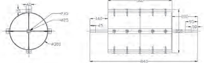
**Fig. 3** Concave 1 and 2 (All dimension are in mm)
