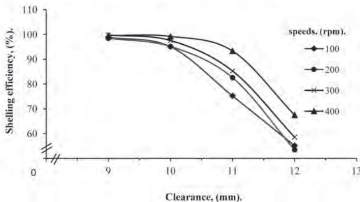
**Fig. 5** Effect of the tested clearance on the shelling efficiency at different speeds
