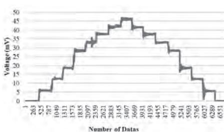
**Fig. 9** Graph showing the linearity of calibration of OAE transducer for vertical force. The obtained equation was: Force (N) = 8.073 + 75.00\* Voltage (mV)
