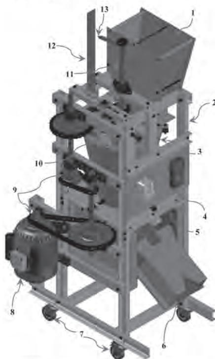
1. Feed hopper, 2. Frame, 3. Shelling chamber, 4. AVO-meter, 5. On/off switch, 6. Discharge outlet, 7. Wheels, 8. Electric motor, 9. Sprocket wheels and chains, 10. Transparent cover, 11. Rotational shaft, 12. Scale of clearance, 13. Pointer
