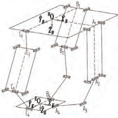
are located in the same plane. It can improve the force of the chain and get partial input-output decoupling.
