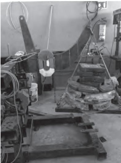
**Fig. 5** Calibration of the transducer OAE to determine vertical force constant
