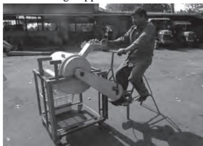
operated arecanut dehusker is shown in **Plate 2**. The details about dehusking cylinder and concave are given in **Fig. 2** and **Fig. 3**.
