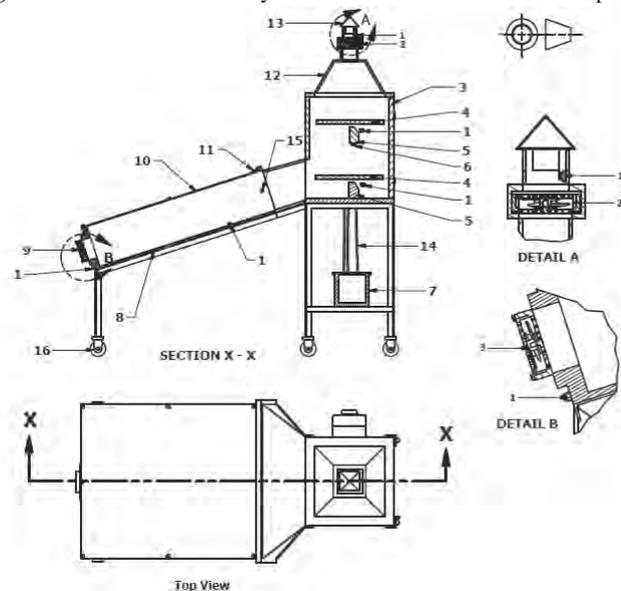
1. Temp./humidity sensors, 2. Exhaust fan, 3. Door frame, 4. Drying racks, 5. Weighing balance, 6. Iron bar (support), 7. Battery/inverter assembly, 8. Solar collector, 9. Inlet fan, 10. Plain glass, 11. Screw bolt, 12. Drying chamber hood, 13. Chimney, 14. Cable, 15. Heating element, 16. Roller
