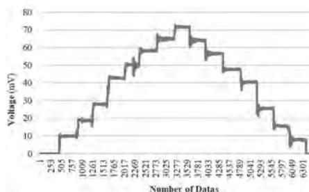
of 0.85 m and **Fig. 13** shows the equation of regression with constant 0.4538 mV N<sup>-1</sup> with a correlation coefficient of the 98.8%. Similar results were obtained by (Campos et al. 2015b) for the calibration of sensors of the type of OAE.
