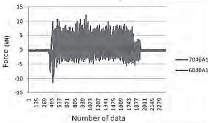
**Fig. 16** Comparative force demand at rigid tine and vibration (amplitude of 0.070 m) to the same depth of 0.40 m and speed of 1.5 km h<sup>-1</sup>. Graph (7040A1) shows the draft force for vibrating tine working at 0.40 m depth. Graph (40A1) shows the draft force for rigid tine working at 0.40 m depth
