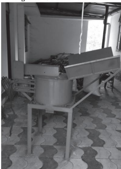
table. While recognizing the importance of the need for powdering the dried manures, Kerala Agricultural University (KAU) has developed a machine named “KAU Manure Pulverizer” to pulverize the dried organic manures such as cow dung, neem cake, biogas slurry, and goat and rabbit fecal pellets etc.
