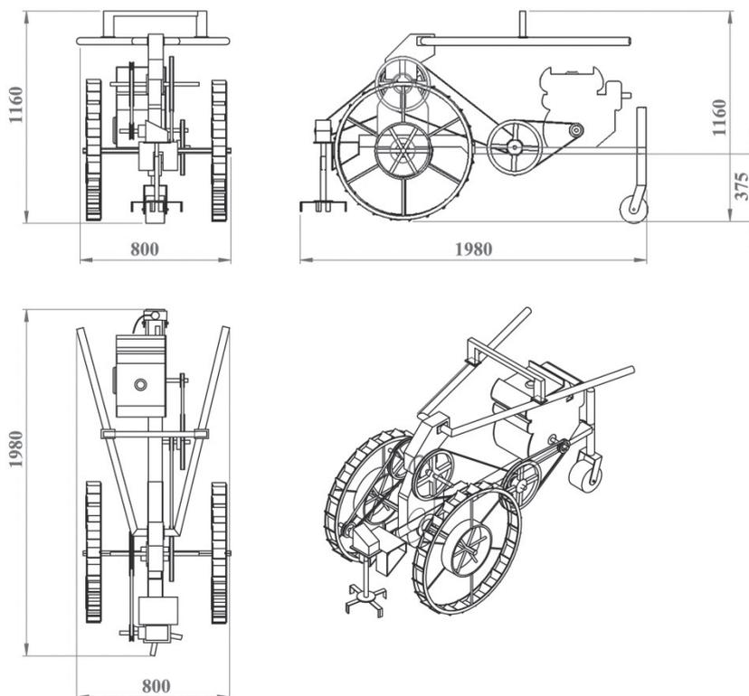
was inserted into a weeding shaft rotating in vertical axis. Adjusting nut was provided to change the pipe position on the weeding rotor shaft. The shaft was mounted on the front end and was supported by a self-aligning bearing.
