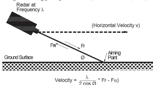
Fig. 2 Installation of radar sensor on a tractor
