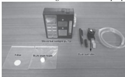
PCXR4 Universal sample pump with IOM dust sampler
