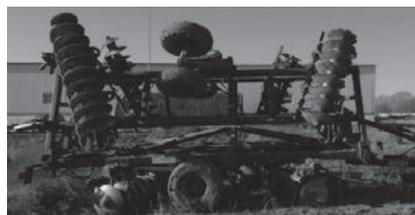
c) – Disc harrow of high-power tractor, working width – 12 m
