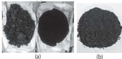
**Fig. 7** Goat fecal pellet powder observed from (a) 5 mm and (b) 10 mm IS sieve sizes
