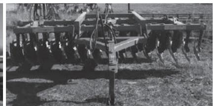
d) – Disc harrow of conventional tractor, working width – 6 m
