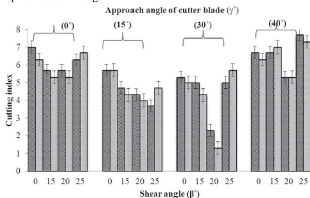
**Fig. 10** Effect of shear angle ( $\beta$ ) on cutting index at selected levels of approach angle ( $\gamma$ ) of cutter blade in impact type pendulum test rig
