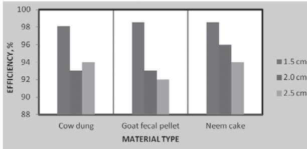
**Fig. 5** Variation of efficiency with clearance at 10 mm sieve size
