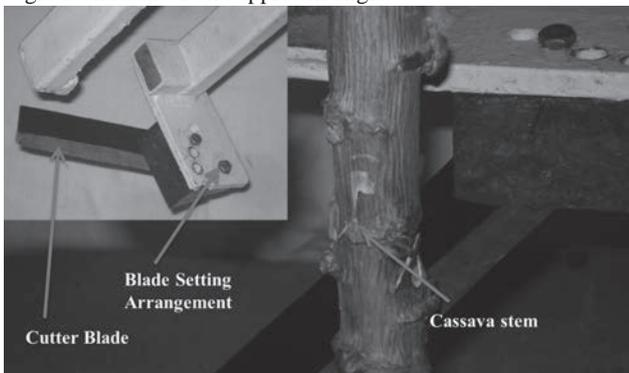
**Fig. 5** Tapered wooden block for adjusting shear and approach angle of cutter blade
