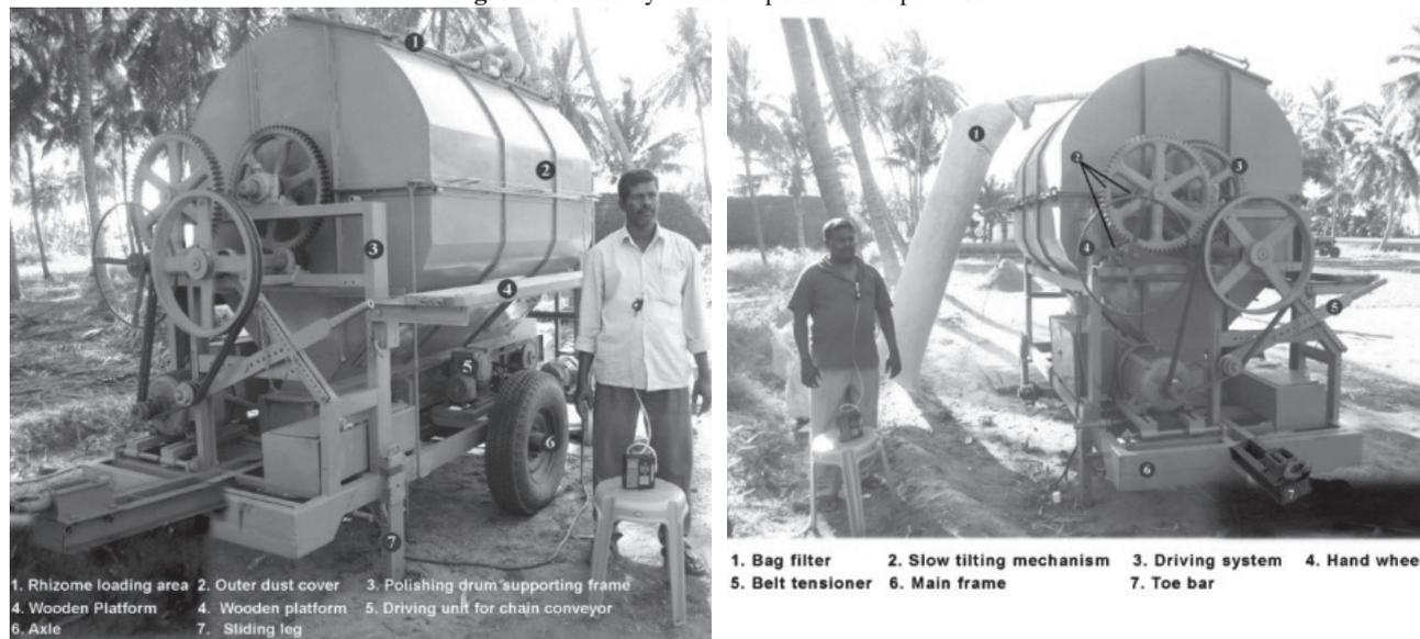
using 50 × 3 mm thick mild steel flat. Seven numbers of 100 × 10 mm size GI bolts were fitted uniformly over each compartment not only to fix the diamond shaped mesh and wire mesh firmly but also to act as an abrasive surface for polishing the
