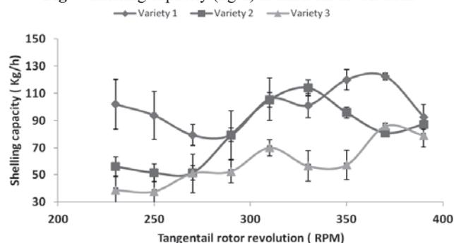
Fig. 6 Shelling efficiency with different revolutions
