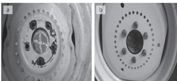
**Fig. 6 a:** Location of hall effect sensor for proximity switching of rear wheels; **b:** Location of hall effect sensor for proximity switching of front wheel
