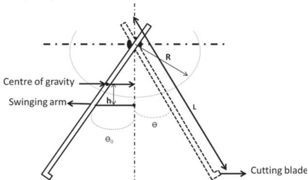
**Fig. 6** Blade Setting arrangement at pendulum hinge point to get desired shear and approach angle
