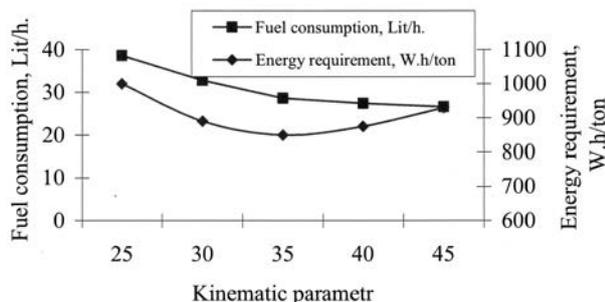
Fig. 6 Effect of kinematic parameter on hourly and turning cost at different pile heights
