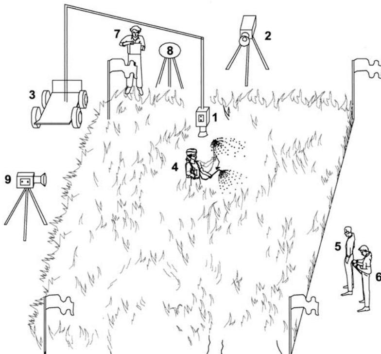
**Legend** 1. Video camera from top, 2. Video camera from side, 3. Moveable elevator vehicle, 4. Spray operator, 5. Lever strokes counter, 6. Time recorders, 7. Person for recording relative humidity (rh), temperature (T), and wind speed (Ws), 8. Try sense device for measuring rh, T, and Ws, 9. Video camera from front
