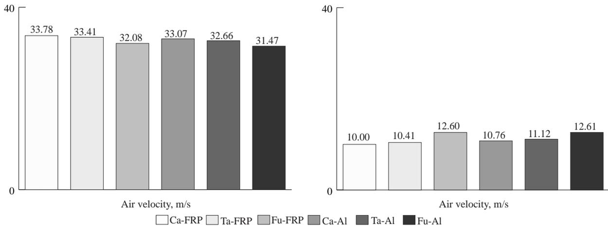
**Fig. 4** Effect of blade stagger angle on (a)air velocity (b)power input to blower
