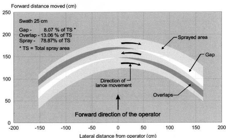
Fig. 8 Variation in amount of spray application in relation to operators and field conditions
