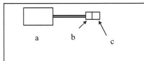
Legend: A. Spray tank, b. Flow meter, c. Pressure gauge, and d. Nozzle
