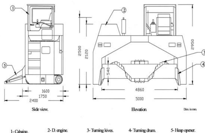
**Fig. 2** Kinematics of compost turning machine
