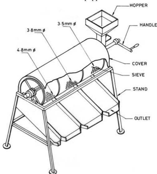
**Fig. 2** Schematics of the cleaner-cum-grader
