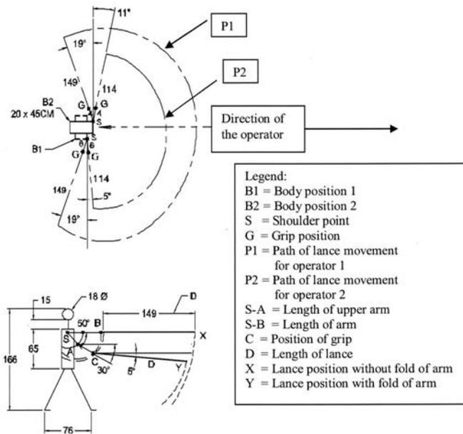
Fig. 6 Changes of nozzle height during horizontal swing of the lance
