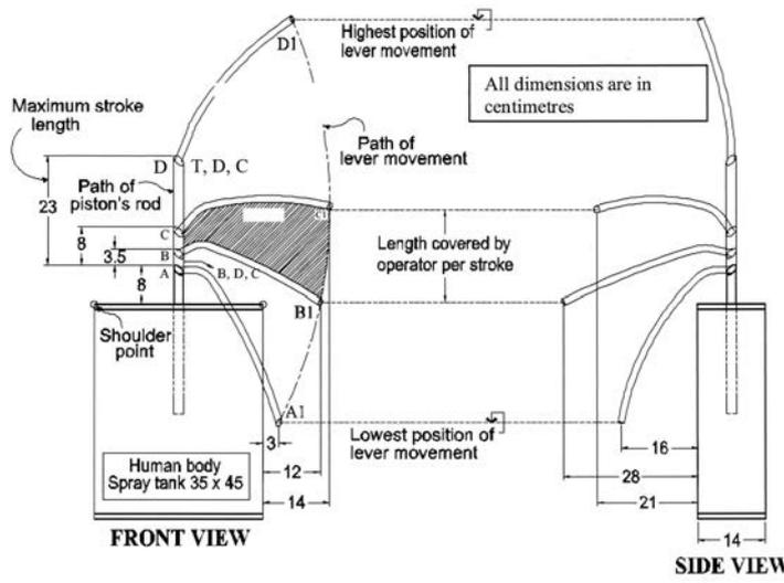
Fig.5 Movement of lance in relation to operator's body; a: Top view, and b: Side view of lane movement
