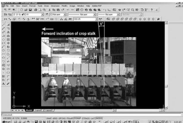
Fig. 3 Inclination of the stalk during the conveying process
