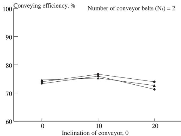
**Fig. 6** Effect of inclination of conveyor on conveying efficiency at selected levels of conveyor belt speed and number of conveyor belts for 2.5 m high maize stalks ( $H_3$ )
