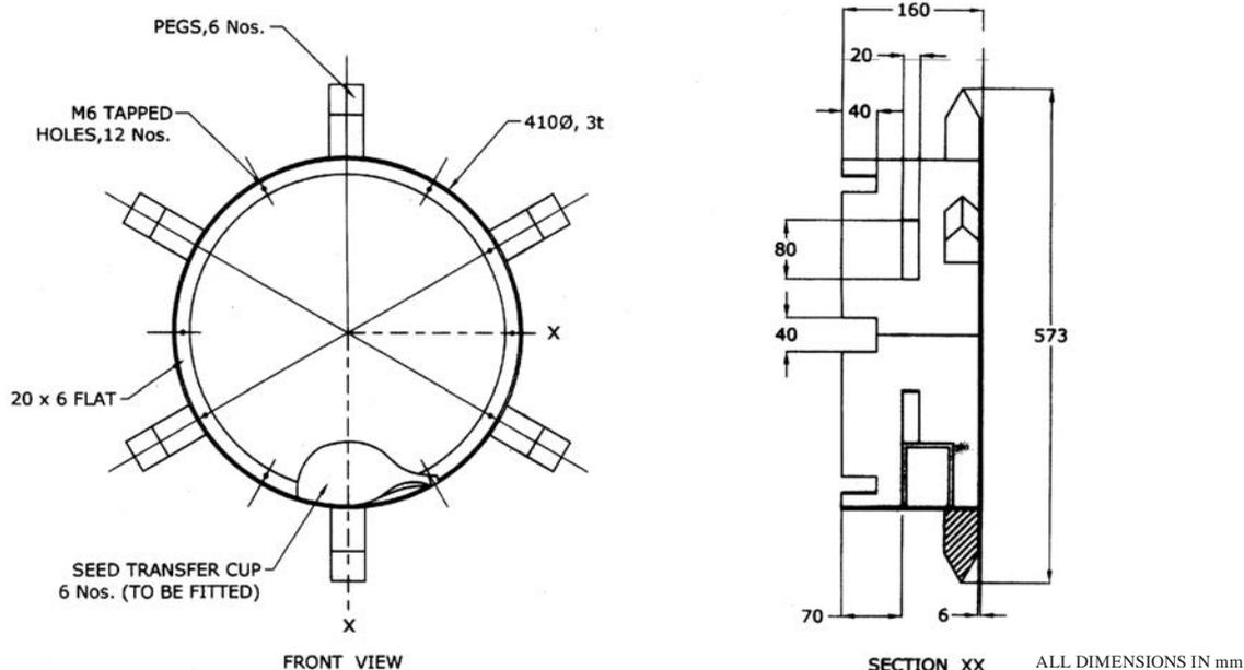
Fig. 5 Prototype dibber wheel
