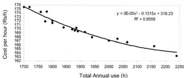
**Fig. 4** Relation between total annual use and cost per hour for 25 hp. tractor
