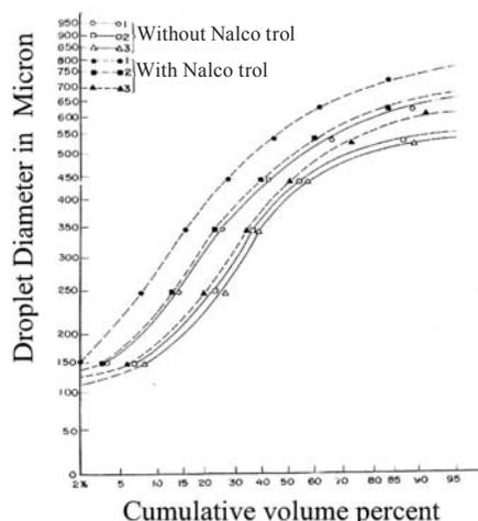
**Fig. 4** Droplet size distribution of Lower leaf surface with aerial spray
