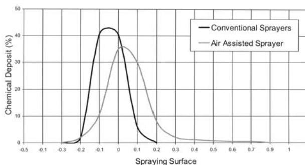
**Fig. 6** Spray coverage on cotton plant canopy with air assisted sleeve boom sprayer and conventional boom sprayer
