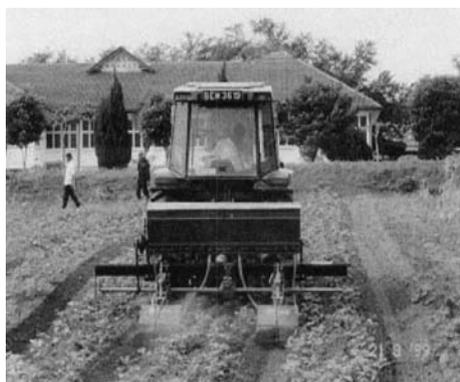
**Fig. 3** Tractor-mounted single-row planter
