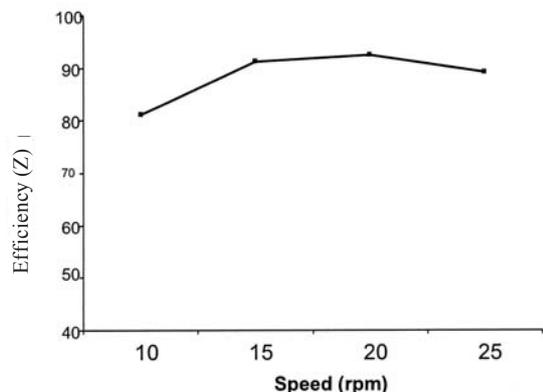
**Fig.5** Effect of speed on overall separation efficiency
