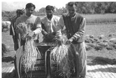
Fig. 3 Motor operated paddy thresher
