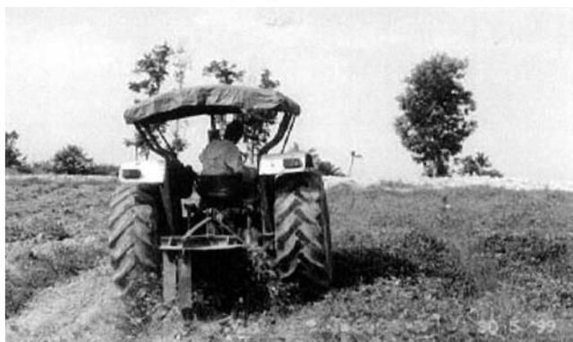
Fig. 8 Root digger-harvester machine
