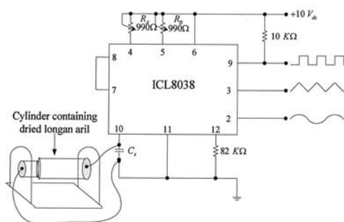
**Fig. 2** The proposed dried longan aril-based capacitor
