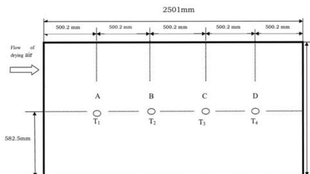
**Fig. 4** Arrangement of thermocouples for sensing drying air temperature just below the agricultural materials
