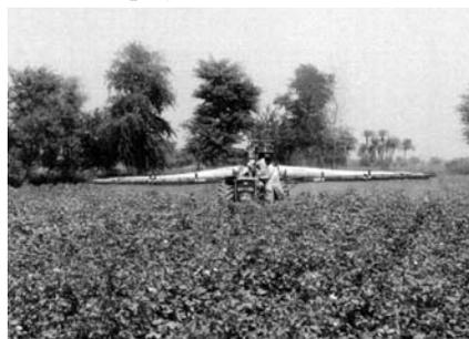
**Fig. 4** Side folding of sleeve boom due to obstruction in the field
