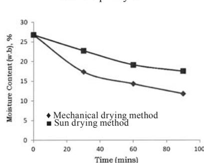
**Table 3** Moisture content readings obtained during drying of paddy rice
