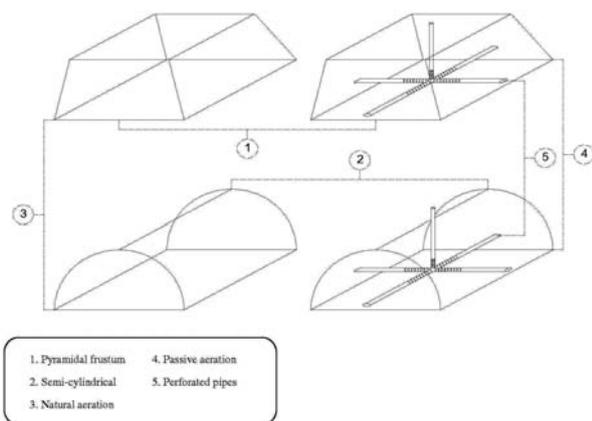
**Figs. 2** A geometrical drawing of the composting piles
