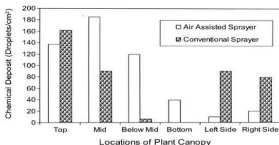
**Fig. 8** Chemical deposit on cotton plant leaves & drift losses with conventional and air assisted boom sprayers
