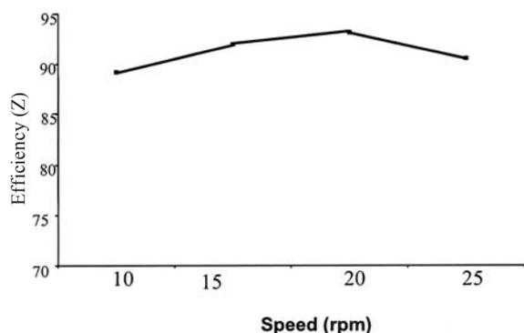
**Fig.4** Effect of speed on separation efficiency for W<sub>2</sub> (61-120 gm)
