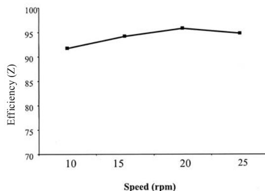
**Fig.5** Effect of speed on separation efficiency for W<sub>3</sub> (> 120 gm)
