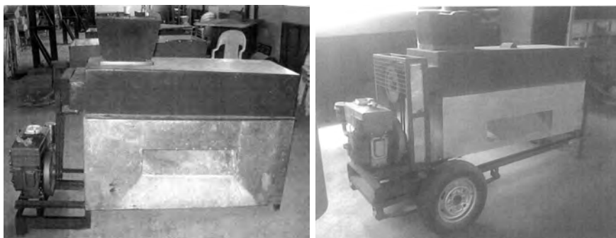
Fig. 7 Pictorial view of the old version of FATOROY cassava peeling machine the improved version
