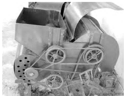
Fig. 2 Constructed and tested Motorized cowpea Thresher (Source Maunde et al. 2010)
