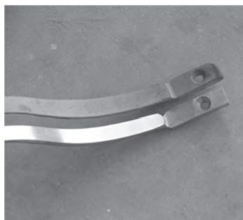
Fig. 5 Improved versus conventional ginning ribs
