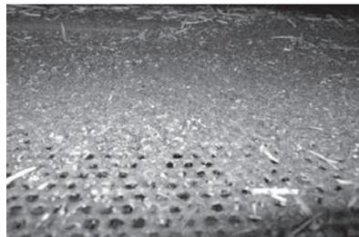
Fig. 16 The adhesion of the rapeseeds cleaning sieve with the smooth surface
