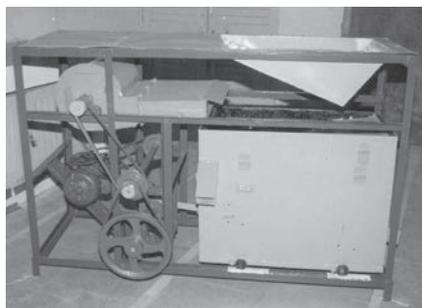
Fig. 2 Developed cumin cleaner cum grader
