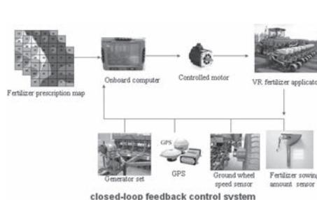
**Fig. 3(b)** Closed-loop Feedback Control System
