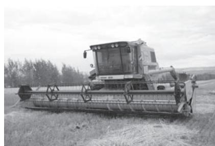
**Fig. 6** Large Intelligent Grain Combine Harvester with 10 kg/s Feed Rate
