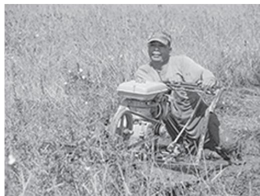
**Fig. 2** The “Laboy” tiller developed by PhilRice and solves the problem of bogging down of tractors in deep mud;
