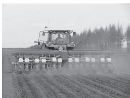
**Fig. 3(a)** Precision Variable Rate Fertilization Seeder
