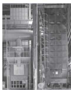
**Fig. 6** Husk furnace paddy dryer
