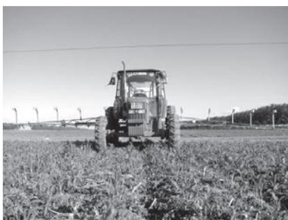
**Fig. 4** IRS Intelligent Targeting Herbicide Sprayer
