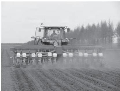
**Fig. 3(a)** Precision Variable Rate Fertilization Seeder
