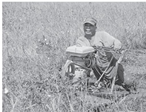
**Fig. 2** The “Laboy” tiller developed by PhilRice and solves the problem of bogging down of tractors in deep mud;
