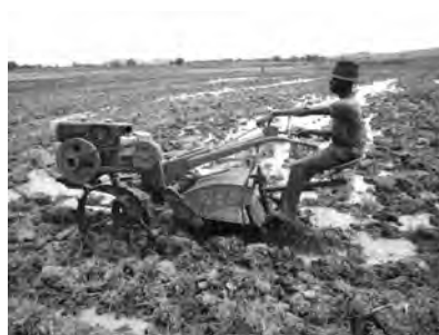
Fig. 6 A Chinese power tiller with a chair working direct puddling, Mbeya region, Jan. 2016
