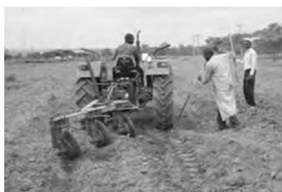
Fig. 7 Wheel slip determination during field evaluation of a tractor (Source: Oni, 2011b)
