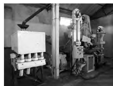
Fig. 14 Small-scale milling plant with paddy separator (Chinese made), Babati, Manyara region, Aug. 2017
