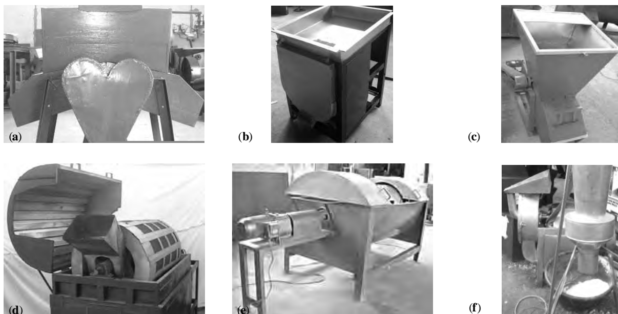
Fig 3 Some cassava processing machineries developed by PRODA (a) double barrel grater (b) chipping machine (c) single barrel grater (d) rotary sieve (e) self-action peeler (f) microniser (Source: www.proda-ng.org )
