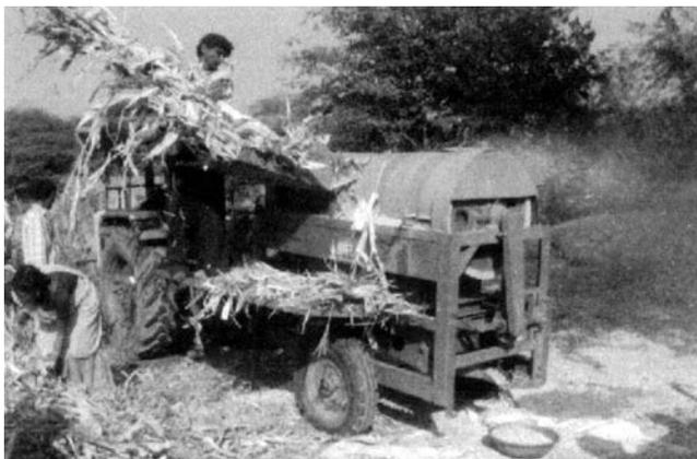
Fig. 10 PAU Design Axial Flow maize Dehusker-Sheller
