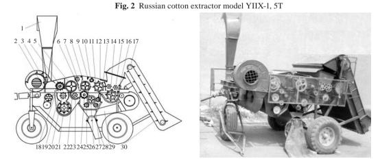
Cotton conveyer, 2. Vacuum valve, 3. Fan, 4/24. Doffing drums, 5/8/26. Saw drums, 6/9/18/22. Shielding, 7. Repelling drum, 10. Blade drum, 11. Shelling drum, 12. Shelling concave, 13/19/22. Net, 14. Impurity remover, 15. Feeder roller, 16. Impurity remover net, 17. Mechanical loader, 20, 21. Strip drums, 23. Small sprocket drum, 27. Rubbing drum, 28. Impurity remover hose, 29. Air duct, 30. Collapsible loader section
