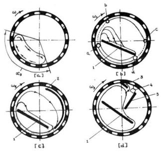
Fig. 3 Developed cleaner-cum-grader for cumin seed
