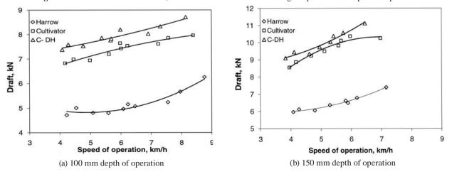
Fig. 3 Variation of draft of cultivator, offset disk harrow and C-DH tillage implement with speed of operation
