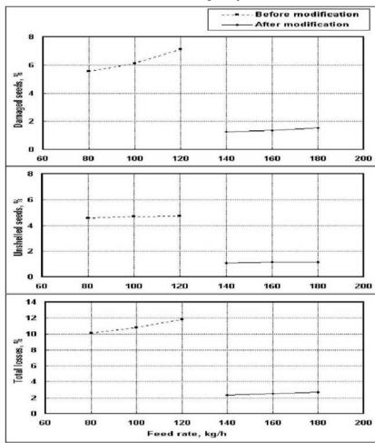
Fig. 5 Effect of feeding rate on damaged, unshelled seeds and tatal losses for the sheller before and after modification at pods moisture content about 17.12 % w.b. and shelling box speed of 1.4 m/s
