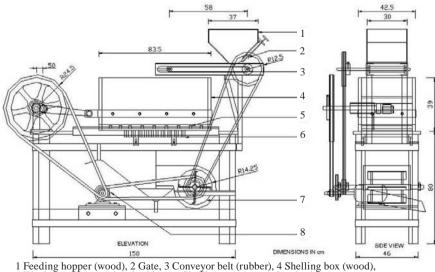
1 Feeding hopper (wood), 2 Gate, 3 Conveyor belt (rubber), 4 Shelling box (wood), 5 Wooken strips (wood and rubber), 6 Shelling screen (wood and rubber), 5 Wooken strips (wood and russer 7 Blower (metal), 8 Electric motor
