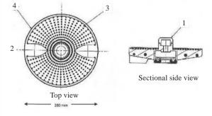
1 = Peeling drum; 2 = Removable inlet cover; 3 = Peeling side surface; 4 = Sliding discharge cover; 5 = Discharge chute for peeled multiplier onion; 6 = Circular base plate
