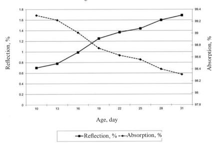
Fig. 4 Reflection and absorption percentages of green beans using He-Ne laser 543.5nm
