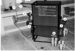
Feed hopper, 2. Main shaft, 3. Gear box, 4. Cleaned seed outlet, 5. Partially cleaned seed outlet, 6. Impurities outlet, 7. Energy meter
