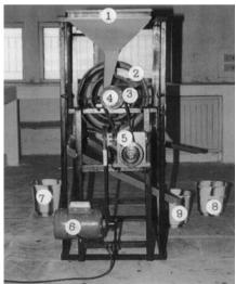
Feed hopper, 2. Outer screen, 3. Inner screen, 4. Main shaft, 5. Gear box,
