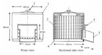
Fig. 3 Front view and sectional cross view of the peeling drum
