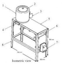
1 = Peeling chamber; 2 = Removable inlet cover; 3 = Discharge chute for peeled multiplier onion; 4 =Outlet for peeled skin; 5 = Working platform; 6 = Motor; 7 = Starter; 8 = Outer frame
