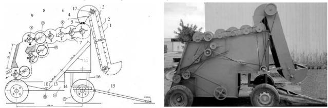
1. Mechanical loader, 2. Chain conveyer, 3. Strip, 4. Tank, 5. Feeder roller, 6. Impact drum, 7. Concave, 8. Saw drum, 9. Doffing drum, 10. Trash auger, 11. Division, 12. Inclined surface, 13. Frame body, 14. Wheels, 15. Hitch point, 16. Revolving circle
