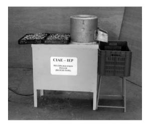
Fig. 6 Performance evaluation of batch type multiplier onion peeler with plastic brushes as abrasive peeling media
