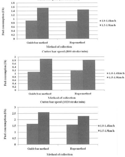
1/h was observed at forward speed between 1.50-1.90 km/h and at cutter bar speed of 1020 Strokes/min. The values of fuel consumption of 0.88 1/h and 0.92 1/h, were at observed at forward speed of 1.00-1.40 km/h and cutter bar speed 550 of strokes/min. The fuel consumption in trench planting was more because two rows of cane were cut at a time and the cane density was more.
