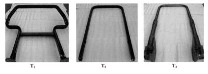
Fig. 2 Geometrical variation in available axle housing of different Indian tractors
