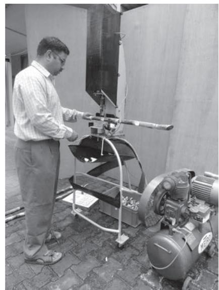
Fig. 5 Pneumatic operated sugarcane bud chipping equipment.
