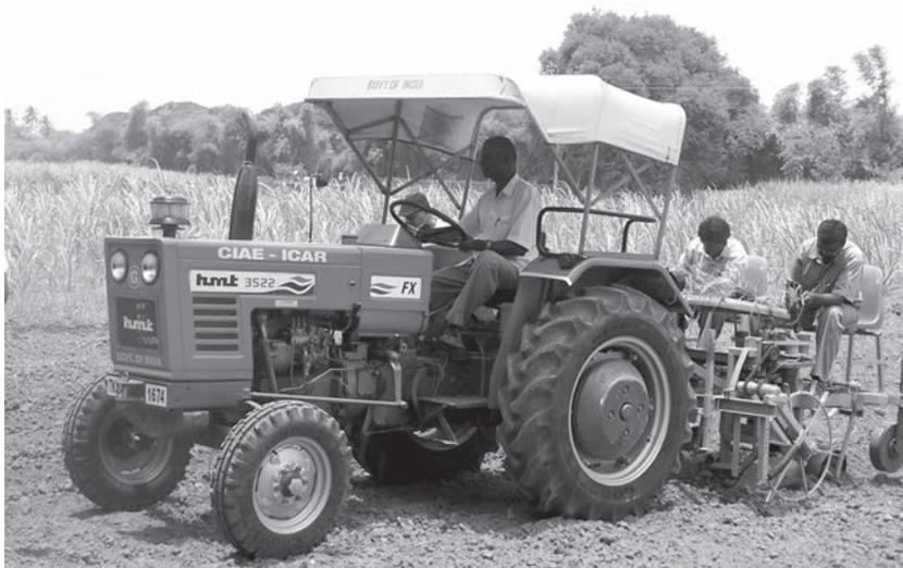
Fig. 6 Field operation of two row tractor drawn mechanical planter for sugarcane bud chip settlings raised in protray (side view).
