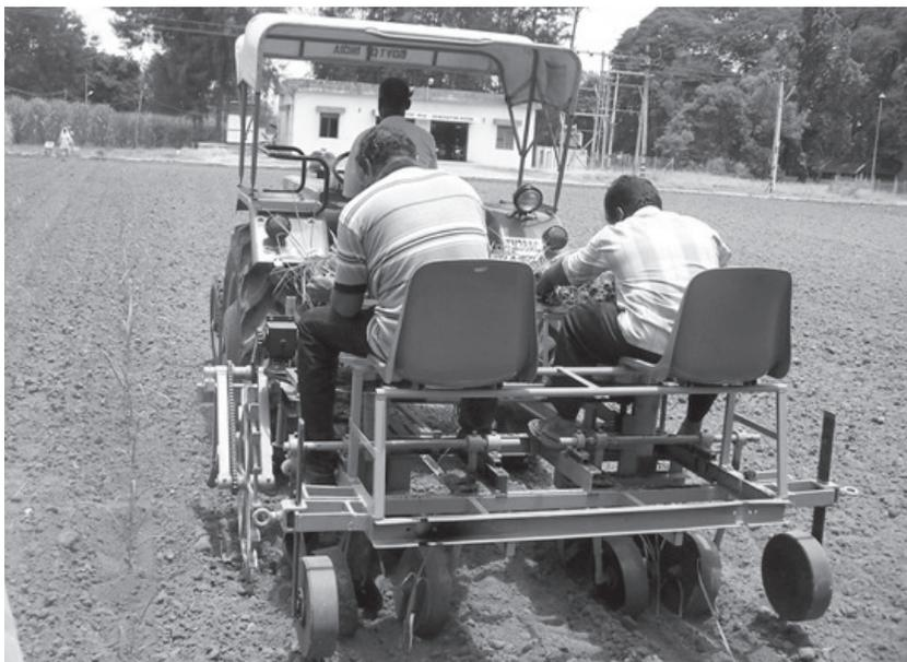
Fig. 7 Field operation of two row tractor drawn mechanical planter for sugarcane bud chip settlings raised in protray (rear view).
