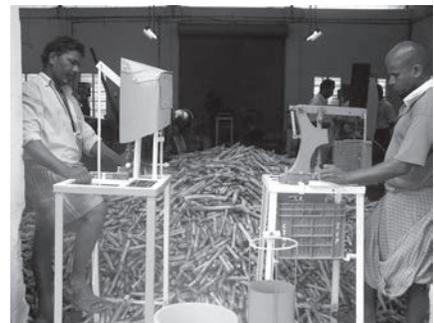
Fig. 4 Pedal operated sugarcane bud chipping equipment.
