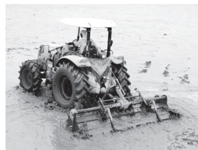
Fig. 13 European brand Tractor 60 hp with Japan brand Rotary Puddler
