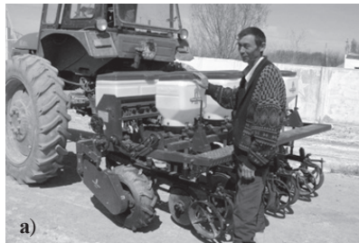
Fig. 5 a) Seeder (no-tillage, new). b) Seed drill (no-tillage, adapted in Cuba) Source: De las Cuevas et al. (2013)
