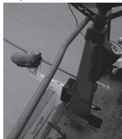
Fig. 3 Video camera installed in front of the combine harvester for imaging the path
