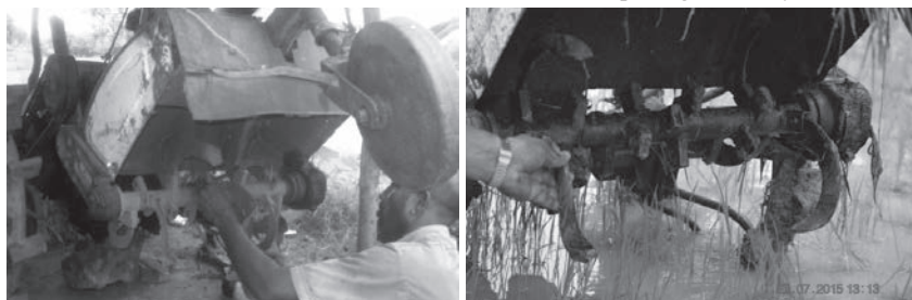
Fig. 3 Arrangements of blade unit in rotary unit of power tiller
