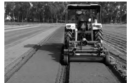
Fig. 5 Rotary tiller cum bed former in operation
