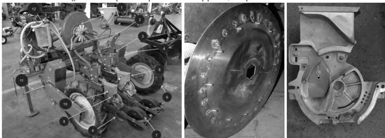
1. Air intake of suction fan, 2. 35 mm suction pipe, 3. Crank to adjust seed depth, 4. Gear box, 5. Seed hopper, 6. Drive wheel, 7. Press wheel, 8. Flapper, 9. Inner singulator, 10. Outer singulator, 11. Transmission hexagon, 12. Seed recovery container
