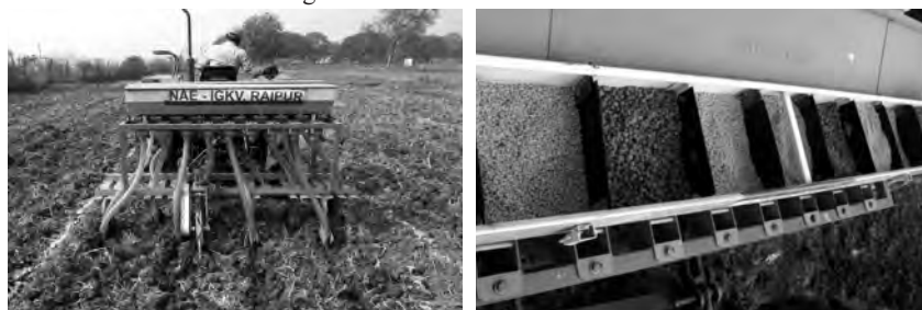
Fig. 5 Sowing of wheat-chickpea (2:1) intercrop by using modified seed cum fertilizer drill
