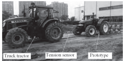
Fig. 4 Measurement schemes of tillage resistances
