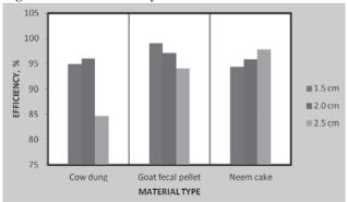
to pulverizer efficiency. The average capacity of the pulverizer was observed to be 500.00 kg h<sup>-1</sup>. **Table 1** presents the efficiency results obtained for the pulverizer using different moisture contents of manures.
