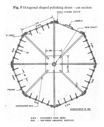
abrasive surface was made by punching 16 gauge mild steel sheets using special 6 mm size punching tool at 25 mm spacing after forming
