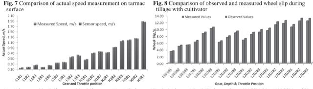
L1 = 1<sup>st</sup> low gear; L2 =  $2^{nd}$  low gear; L3 =  $3^{rd}$  low gear; H1 = 1<sup>st</sup> high gear; H2 =  $2^{nd}$  high gear; H3 =  $3^{rd}$  high gear; R1 = 1000 RPM; R2 = 1500 RPM; and R3 = 2000 RPM
