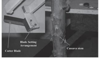
Fig. 5 Tapered wooden block for adjusting shear and approach angle of cutter blade  $% \left( {{{\mathbf{F}}_{i}}} \right)$
