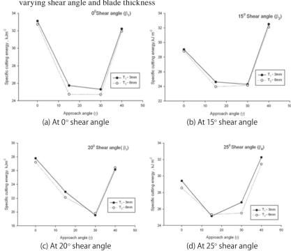
Fig. 7 Effect of approach angle on specific cutting energy of cassava stem with varying shear angle and blade thickness
