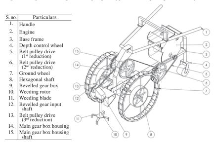
Fig. 1 Conceptual drawing of developed prototype weeder depicting all the components
