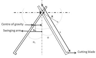
Fig. 6 Blade Setting arrangement at pendulum hinge point to get desired shear and approach angle
