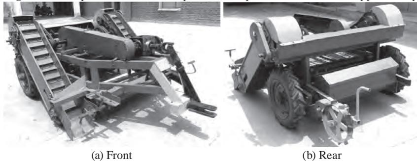
**Fig. 4** A view of tractor-operated seeder for mat type paddy nursery operational under controlled field conditions
