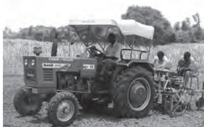
**Fig. 4** Machine for sowing intercrop with sugarcane
