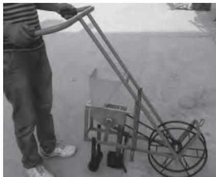
IISR Manual multicrop planter for sowing intercrop in sugarcane
