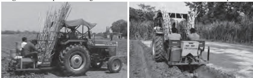
setts etc. A tractor operated double bottom pit digger was developed at IISR, Lucknow for mechanizing ring pit planting of sugarcane (Singh et al., 2017). This machine can dig 150 pits in an hour and saves lots of labour and cost over conventional digging of pits.
