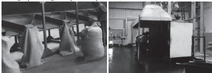
Fig. 11 Chestnuts opening machine and separation of the husk process and almond at Condor Caju Agro processing factory in Gaza province (Source: IAM, 2022)
