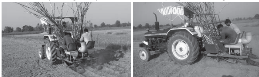
Fig. 2 Sugarcane set as planted in the field by sugarcane cutter planter
